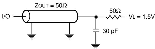
**Figure 1. Output Load**
