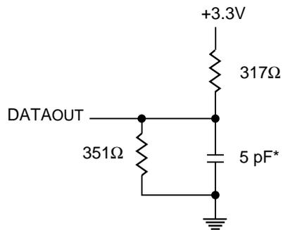
**Figure 2. Output Load**
