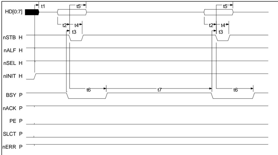
**FIGURE 12 - SPP DATA WRITE TIMING (PARALLEL PORT SIGNALS)**
