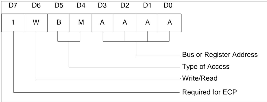
**FIGURE 4 – PARALLEL PORT ADDRESS WRITE AND DATA BITS**
