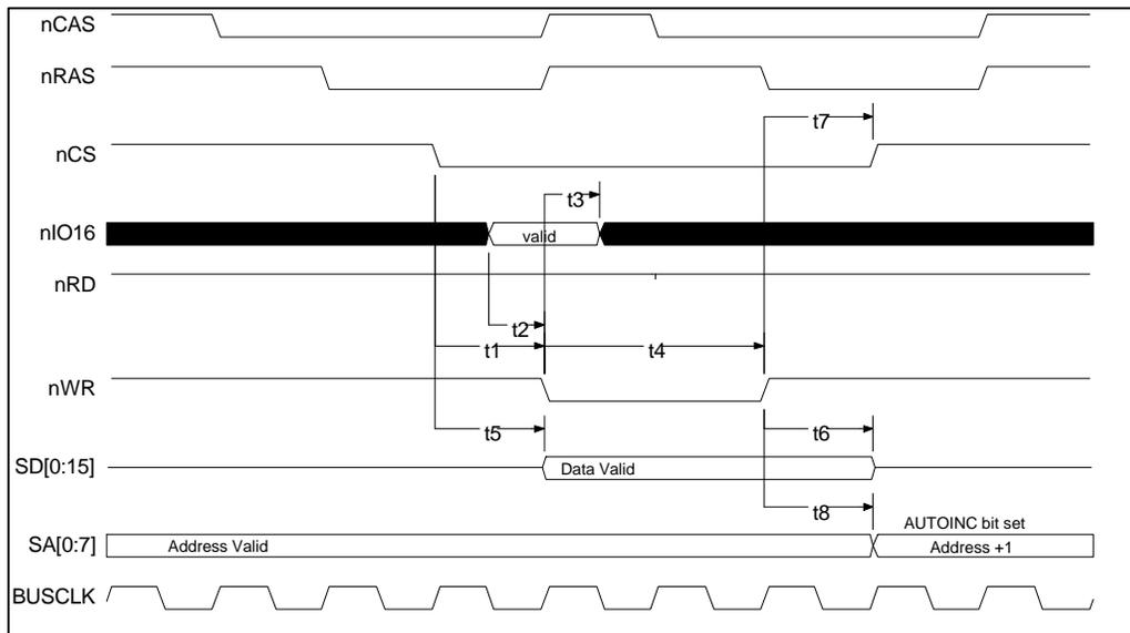
**FIGURE 22 - PERIPHERAL BUS WRITE CYCLE TIMING**
