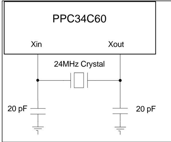
FIGURE 9 - SUGGESTED 24 MHz OSCILLATOR CIRCUIT
