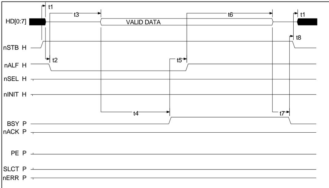
**FIGURE 17 - EPP DATA READ TIMING (PARALLEL PORT SIGNALS)**
