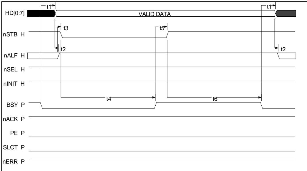
**FIGURE 19 - ECP FORWARD DATA TRANSFER TIMING
