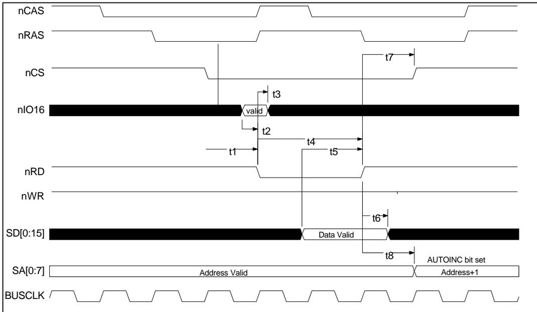
**FIGURE 21 - PERIPHERAL BUS READ CYCLE TIMING**
