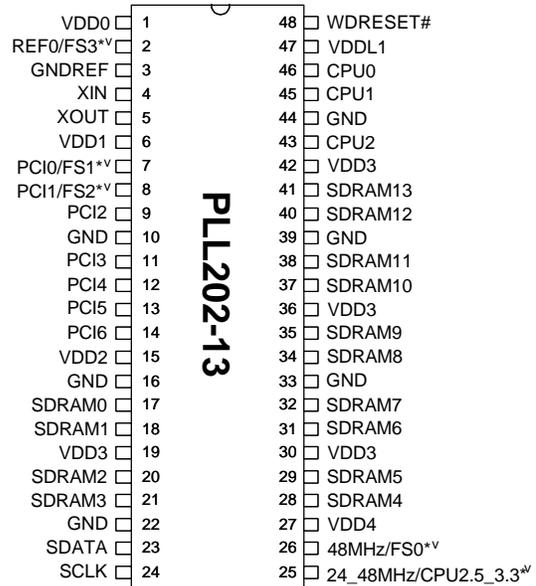
Note: <sup>v</sup>: Pull down, #: Active low \*<sup>w</sup>: Bi-directional latched at power-up
