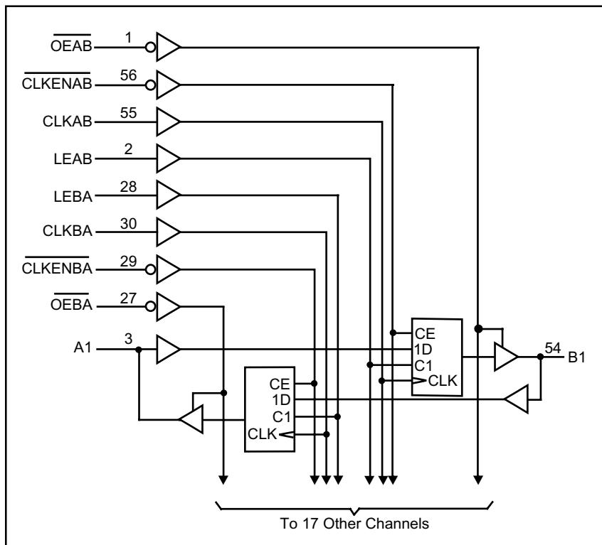
To ensure the high-impedance state during power up or power down, OE should be tied to  $V_{DD}$  through a pull-up resistor; the minimum value of the resistor is determined by the current-sinking capability of the driver.
