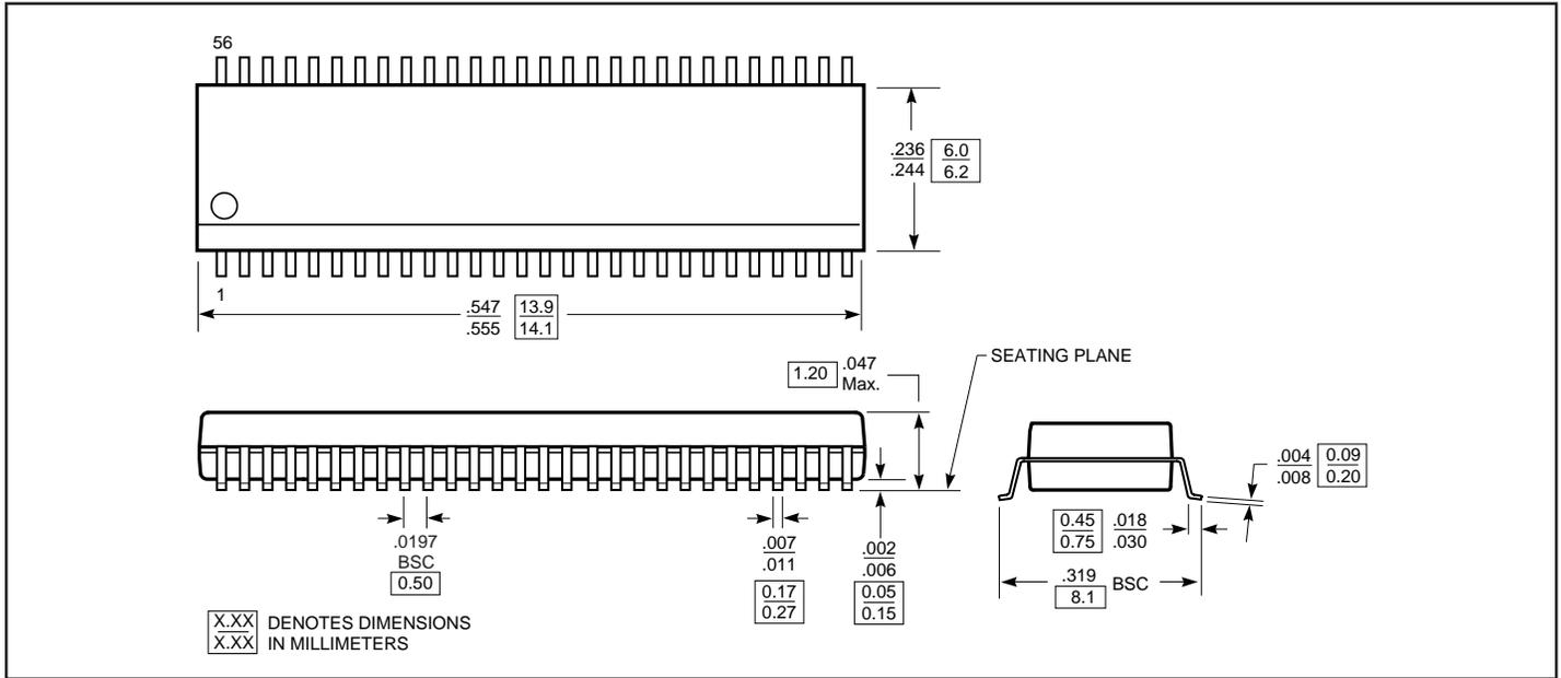
**Packaging Mechanical: 56-Pin SSOP (V) Package**
