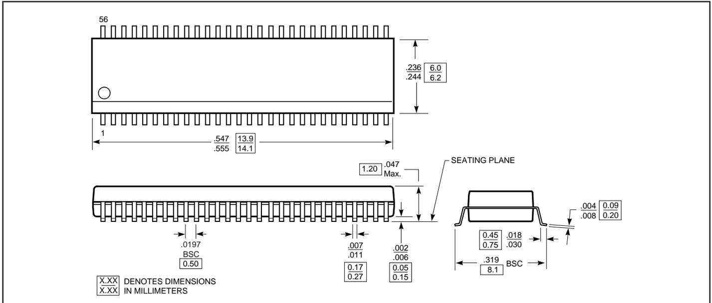
**Packaging Mechanical: 56-Pin SSOP (V) Package**
