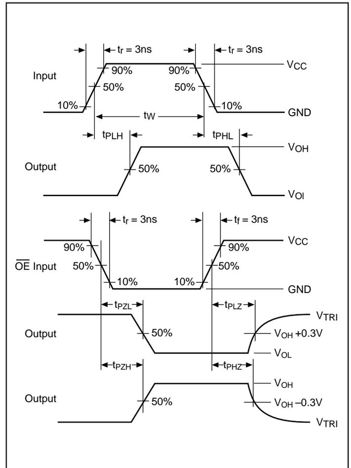
Figure 3. AC Waveforms
