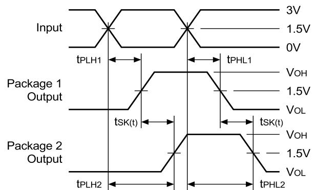
$$t_{SK(t)} = | t_{PLH2} - t_{PLH1} | \text{ or } | t_{PHL2} - t_{PHL1} |$$
