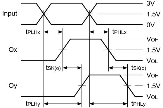
$$t_{SK(o)} = | t_{PLHy} - t_{PLHx} | \text{ or } | t_{PHLy} - t_{PHLx} |$$
