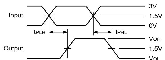
$$t_{SK(p)} = | t_{PHL} - t_{PLH} |$$
