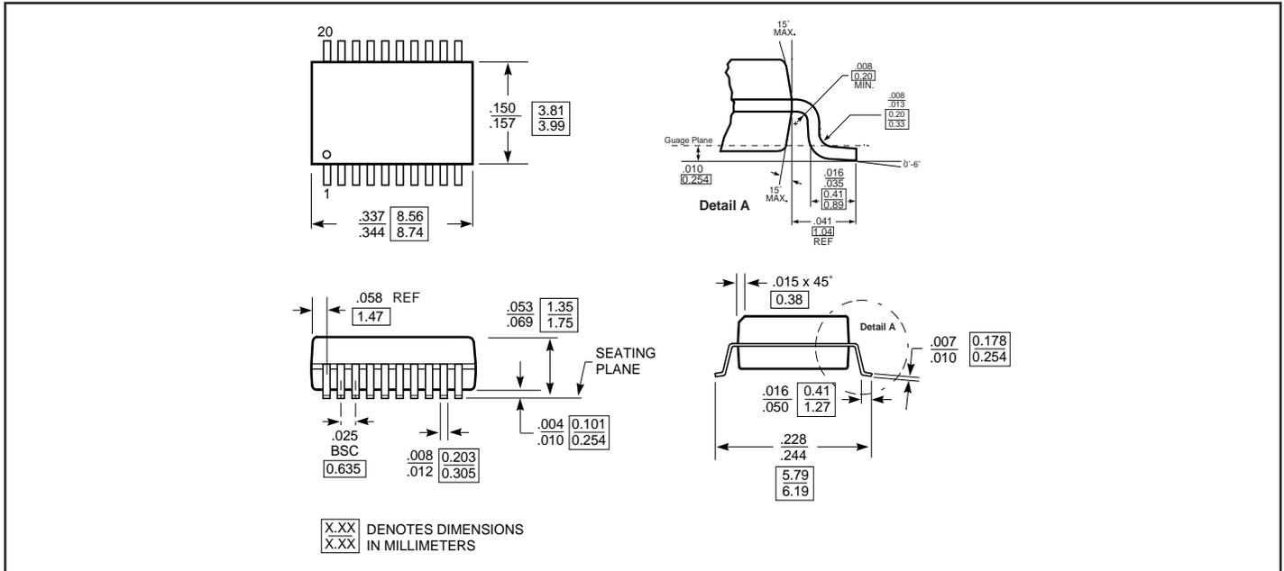
Packaging Mechanical - 20-pin SOIC (S-package)
