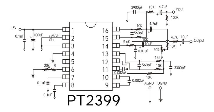
Note: External Resistor having a value of 10 K Ohms to 50 K Ohms may be used. The recommended Resistor Value (R) is 10 K Ohms. When the value of the Resistor (R) increases, the range of the Delay Time also increases.
