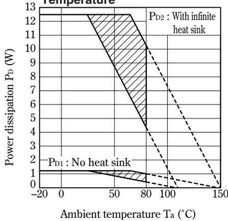
Note) Oblique line portion: Overheat shut down operates in this area
