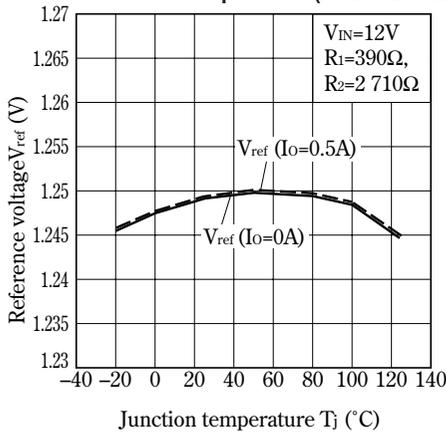
**Fig.7 Reference Voltage Fluctuation vs. Junction Temperature (PQ25VB012FZ)**
