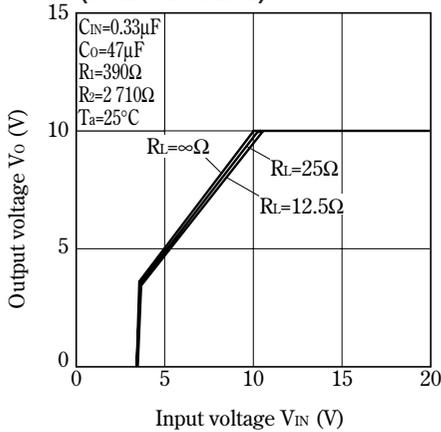
**Fig.9 Output Voltage vs. Input Voltage (PQ25VB012FZ)**
