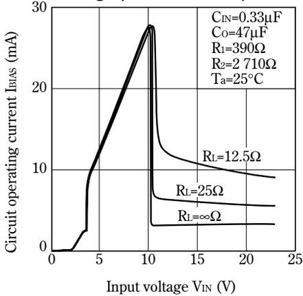
**Fig.11 Circuit Operating Current vs. Input Voltage (PQ25VB012FZ)**
