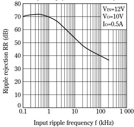
**Fig.17 Ripple Rejection vs. Input Ripple Frequency (PQ25VB012FZ)**
