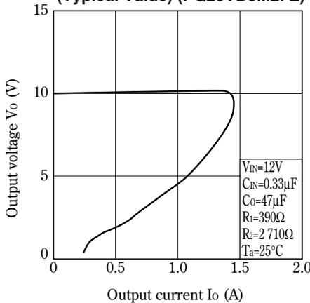
**Fig.5 Overcurrent Protection Characteristics (Typical Value) (PQ25VB012FZ)**
