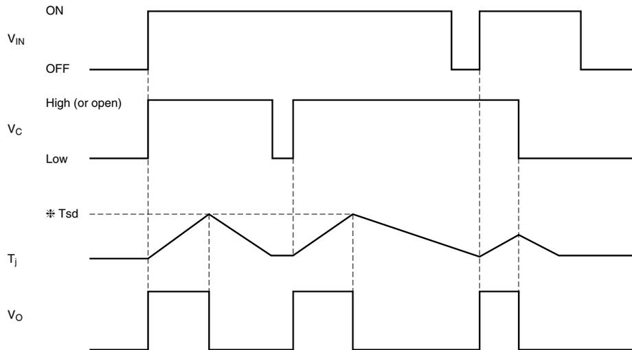
\*Tsd: Overheat shut-down temperature (T<sub>j</sub> ≥ 110°C)
