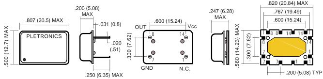
Solder pad layout may use any combination of pins 1, 7, 8 & 14 shown. Recommended pad size is .12 (3.1) x .07 (1.8) typical.
