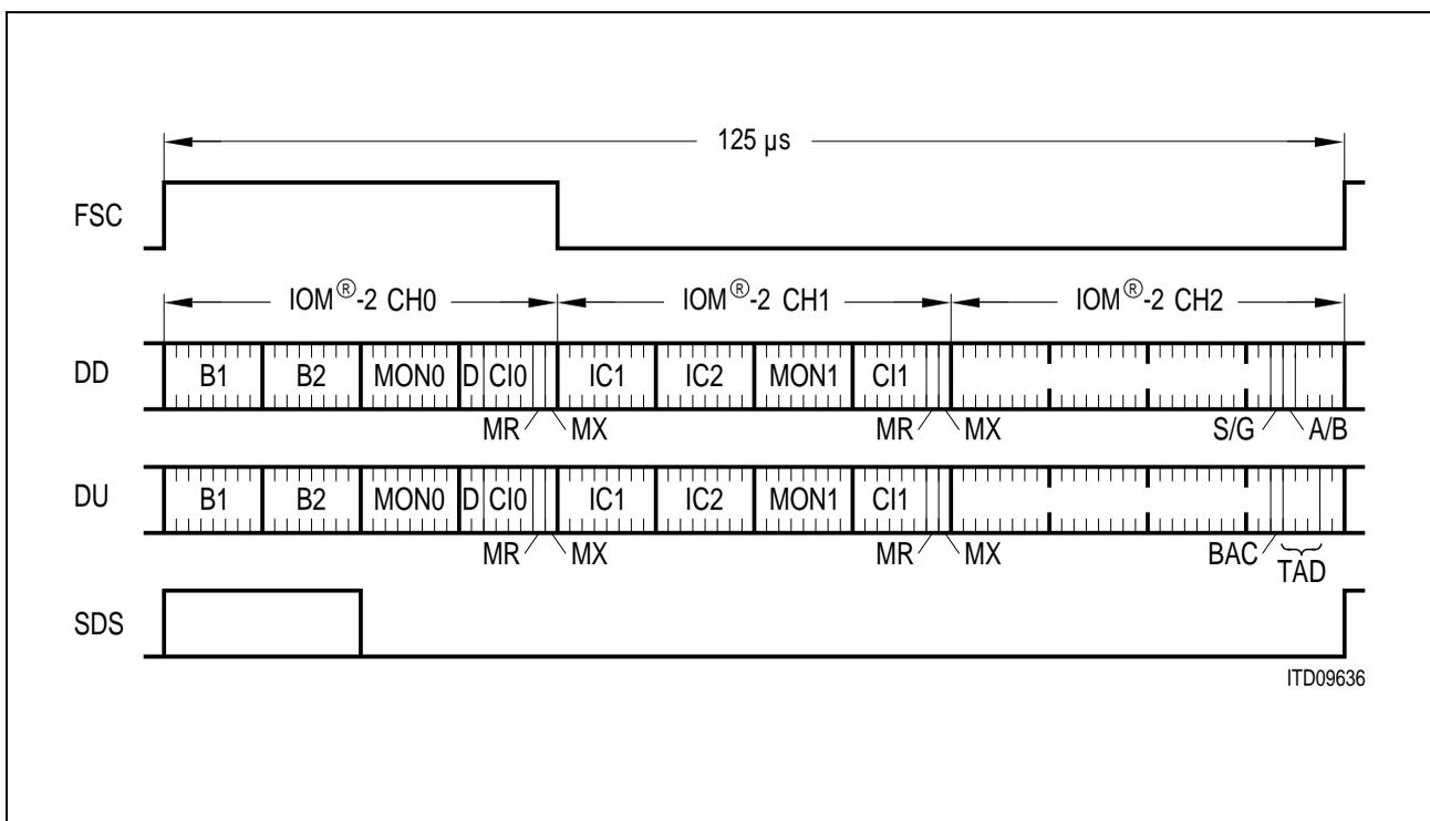
**Figure 53 Definition of IOM<sup>®</sup>-2 Channels in Terminal Timing Mode**
