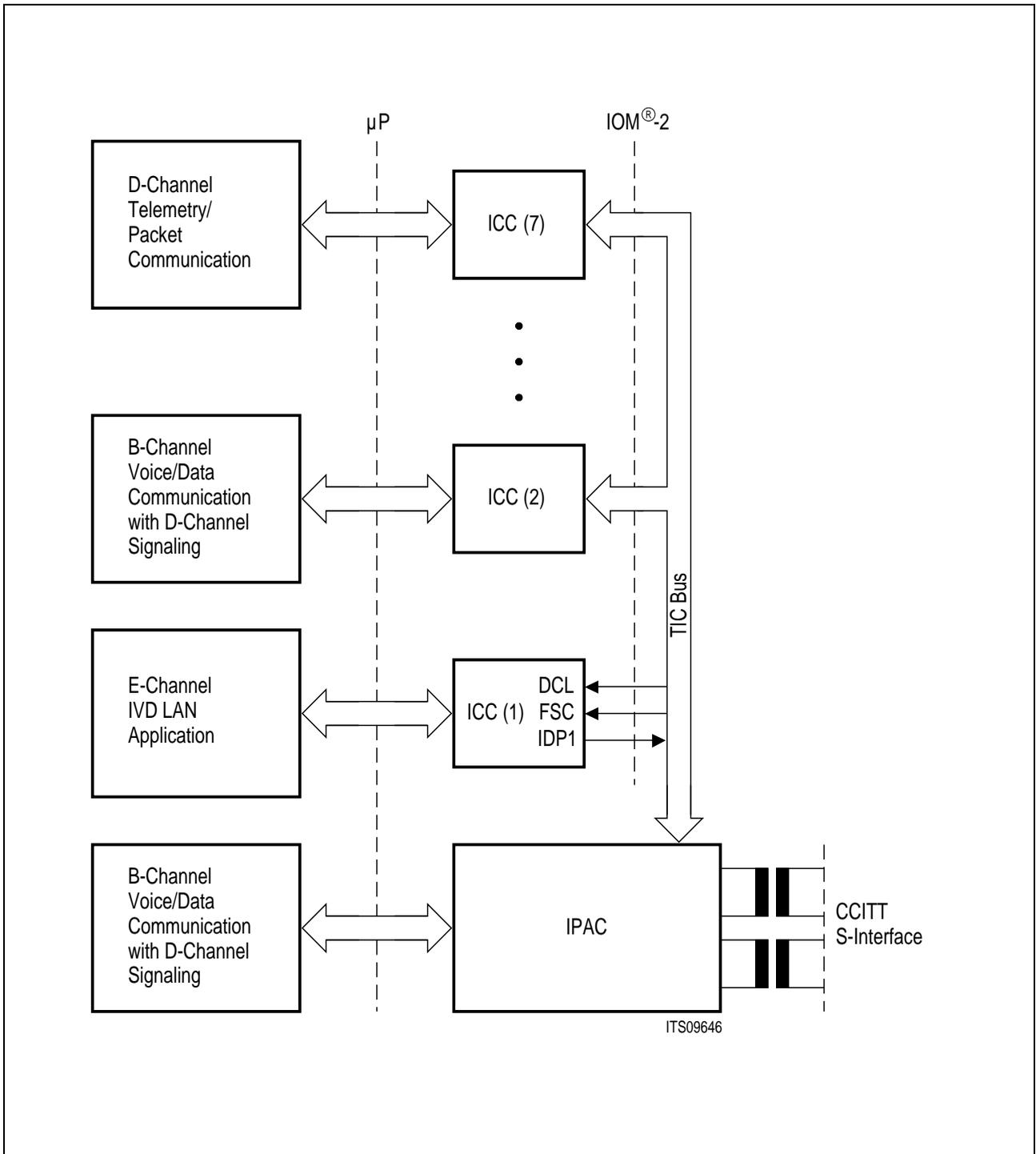
Figure 66 Applications of TIC Bus in IOM<sup>®</sup>-2 Bus Configuration
