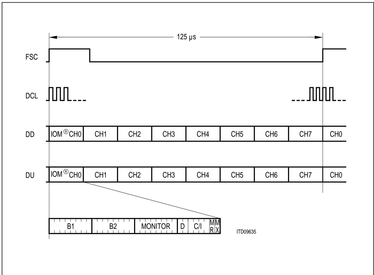
**Figure 52    Multiplexed Frame Structure of the IOM<sup>®</sup>-2 Interface in Non-TE Timing Mode**
