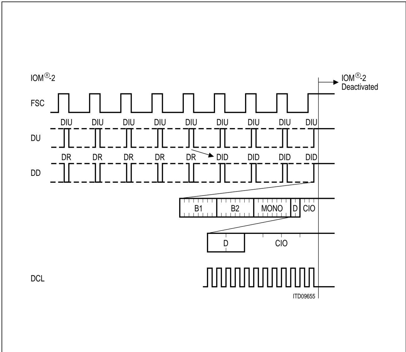
**Figure 90 Deactivation of the IOM<sup>®</sup> Interface**
