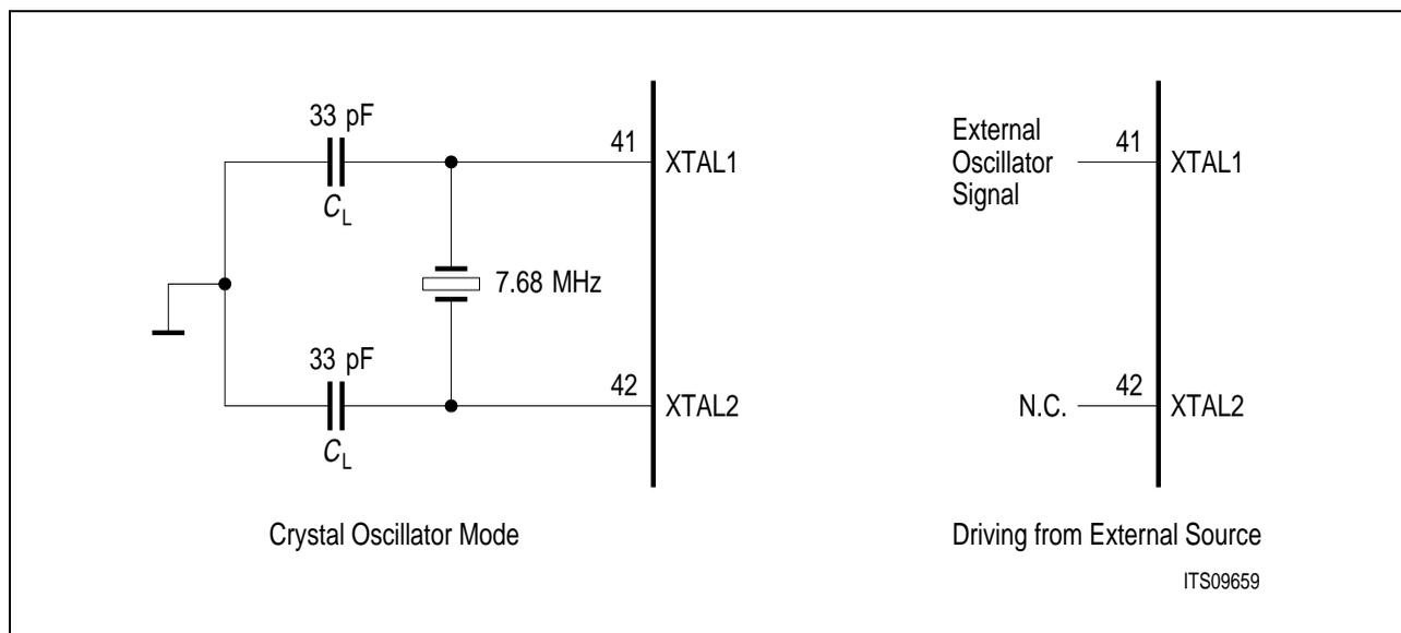
Figure 101 Oscillator Circuits
