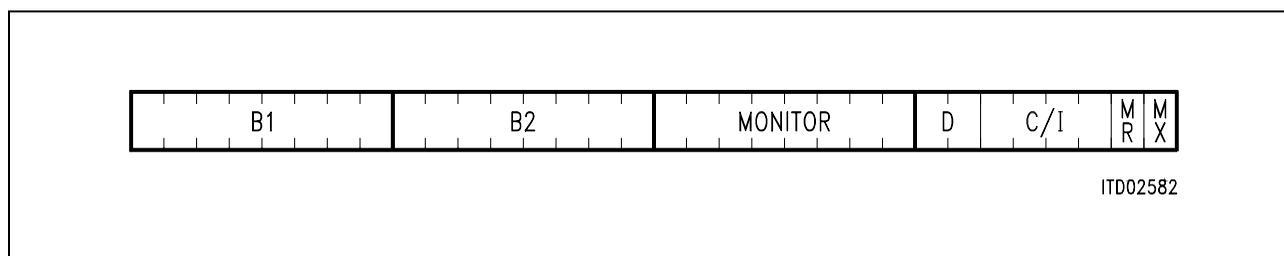
**Figure 51 Channel Structure of IOM<sup>®</sup>-2**
