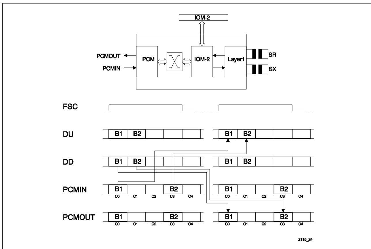
**Figure 72 Switching Data between PCM and IOM<sup>®</sup>-2**
