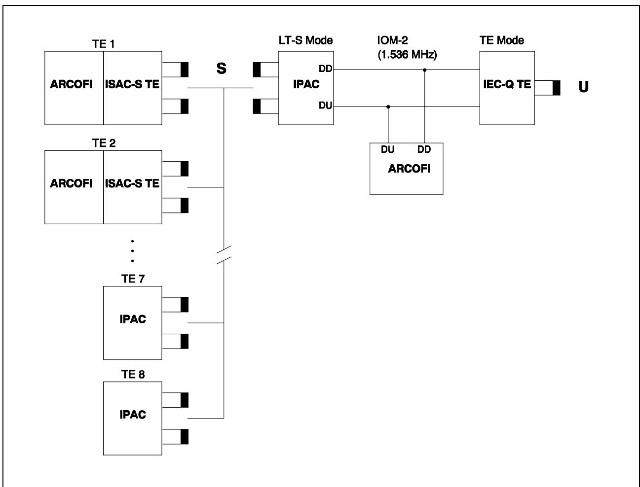
Figure 20 Intelligent NT-Configuration for IOM<sup>®</sup>-2 Channel Switching
