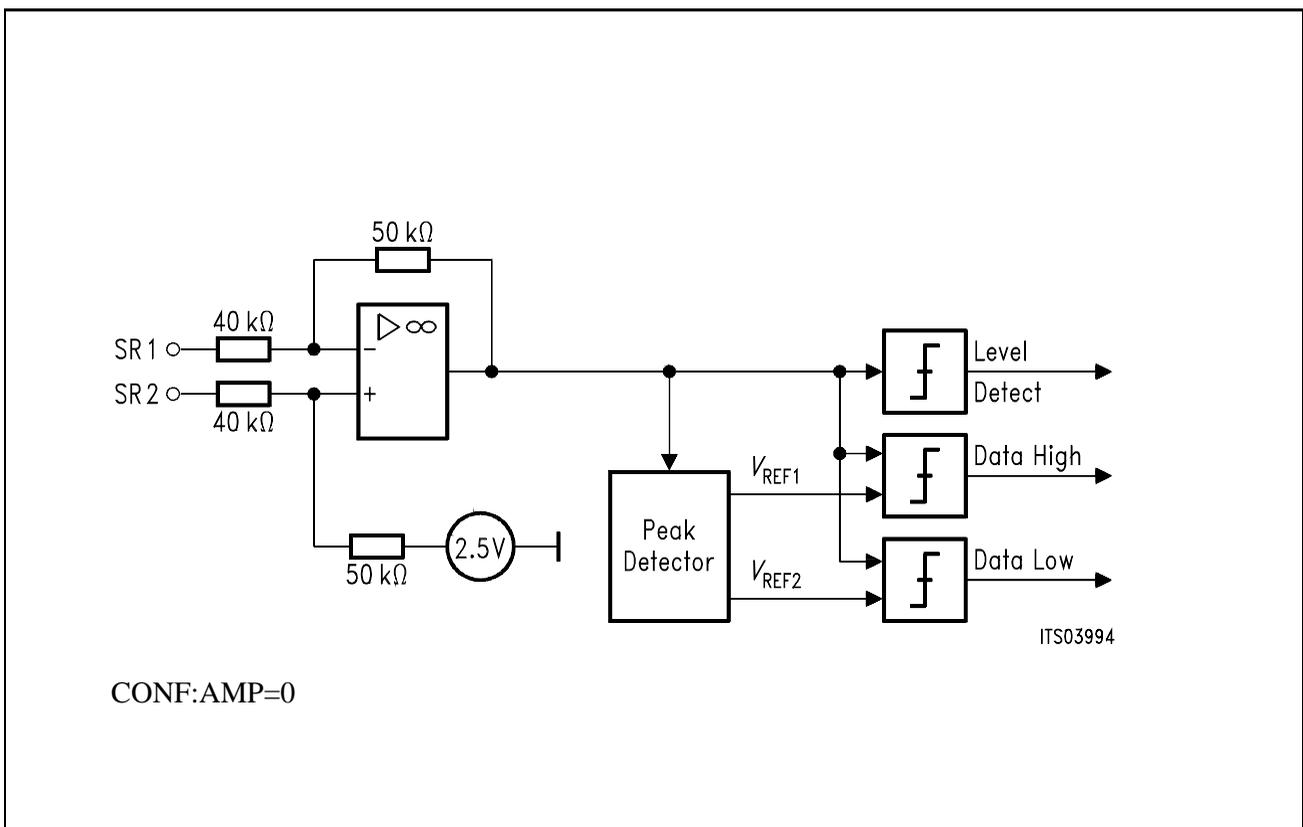
Figure 29 Receiver Circuit
