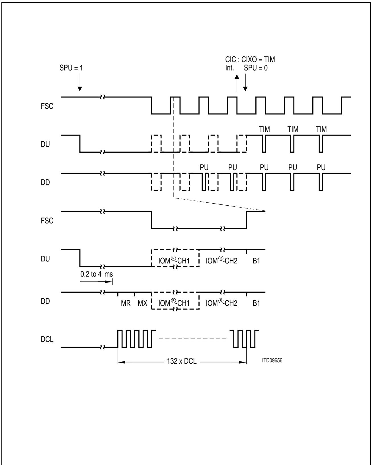
Figure 91 Activation of the IOM<sup>®</sup> interface
