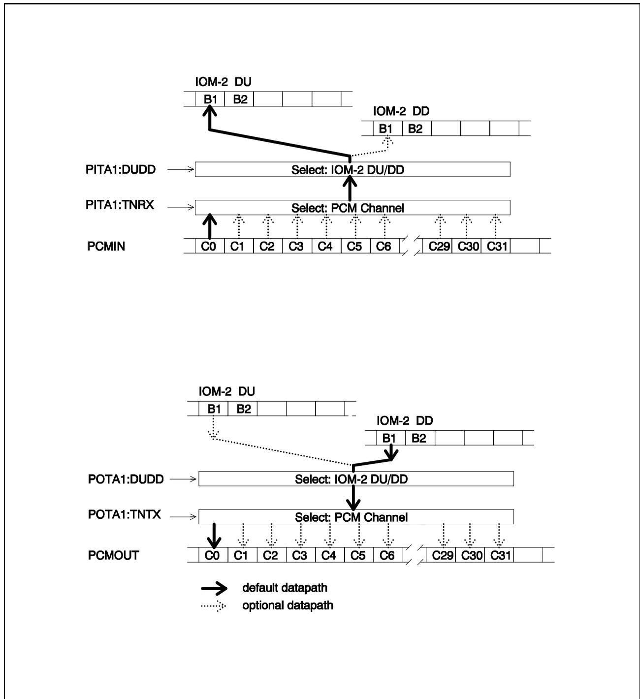
Figure 76 Switching of PCM Timeslots on IOM<sup>®</sup>-2 Channel B1
