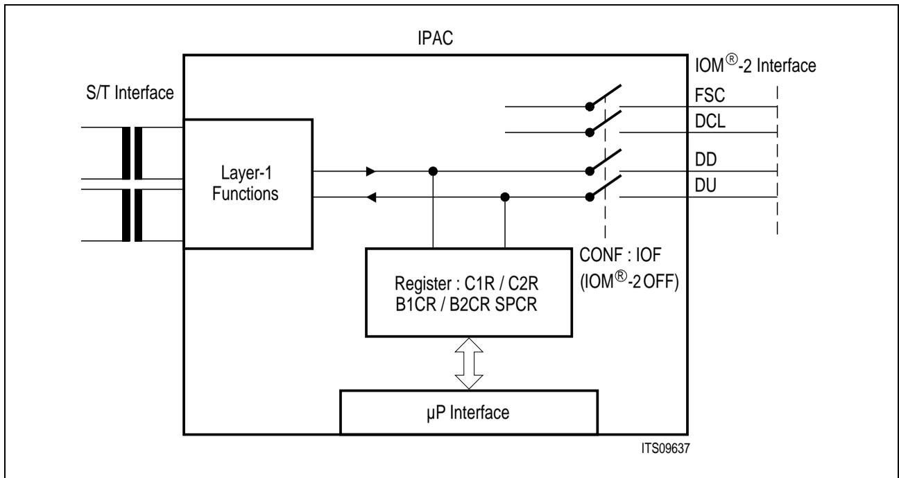
Figure 60 Principle of B/IC Channel Access in IOM<sup>®</sup>-2 Terminal Mode
