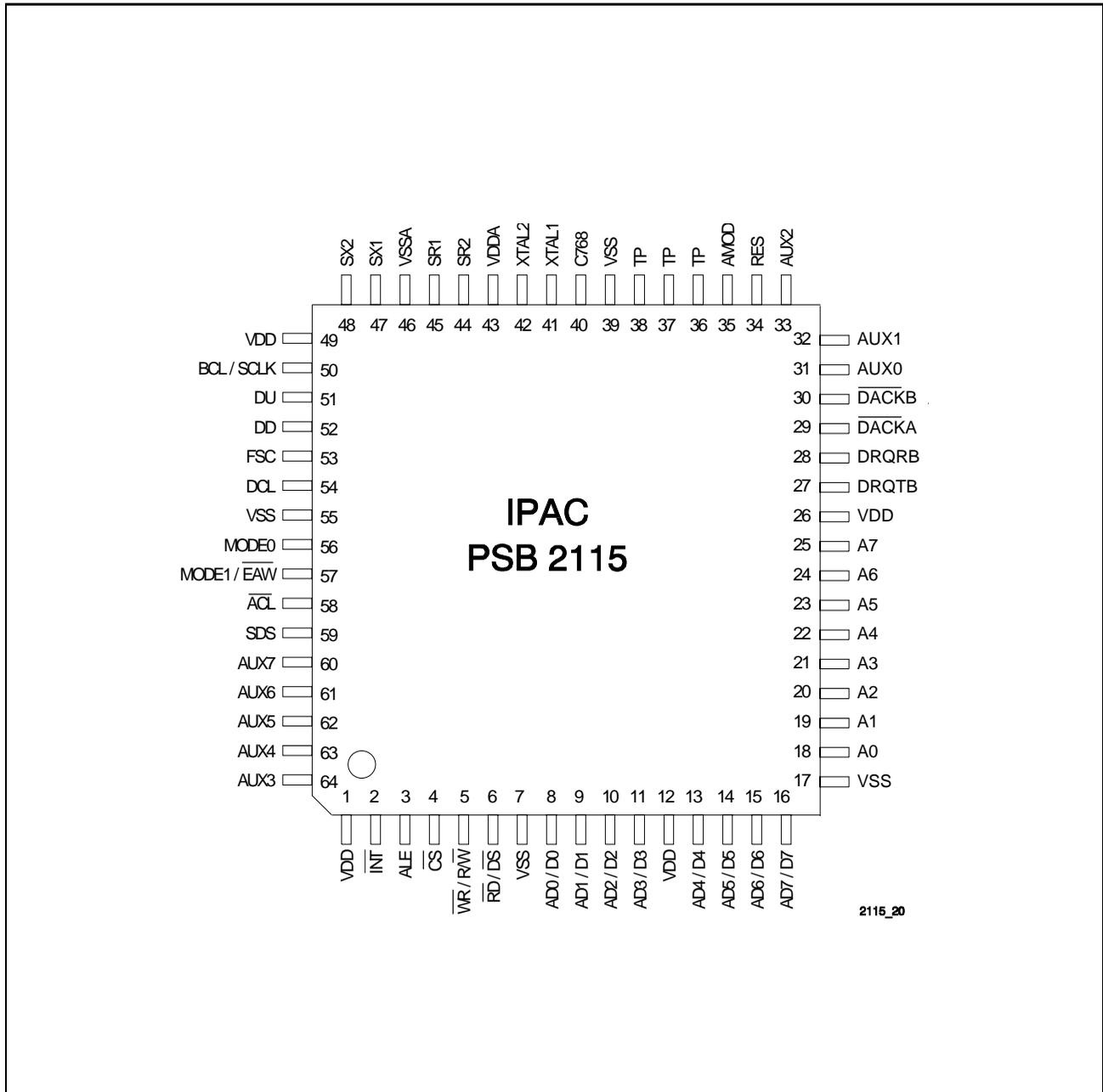
Figure 2 Pin Configuration
