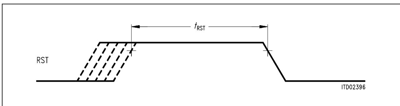
**Figure 118 Reset Signal**
