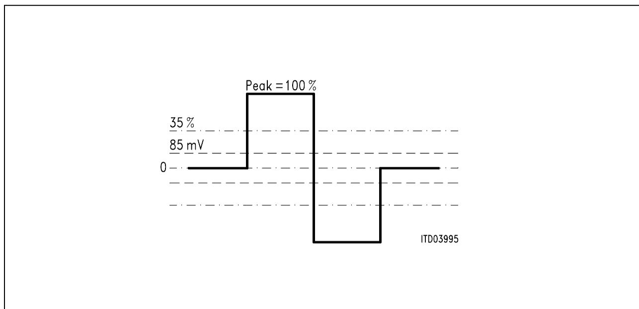
**Figure 30 Receiver Thresholds**
