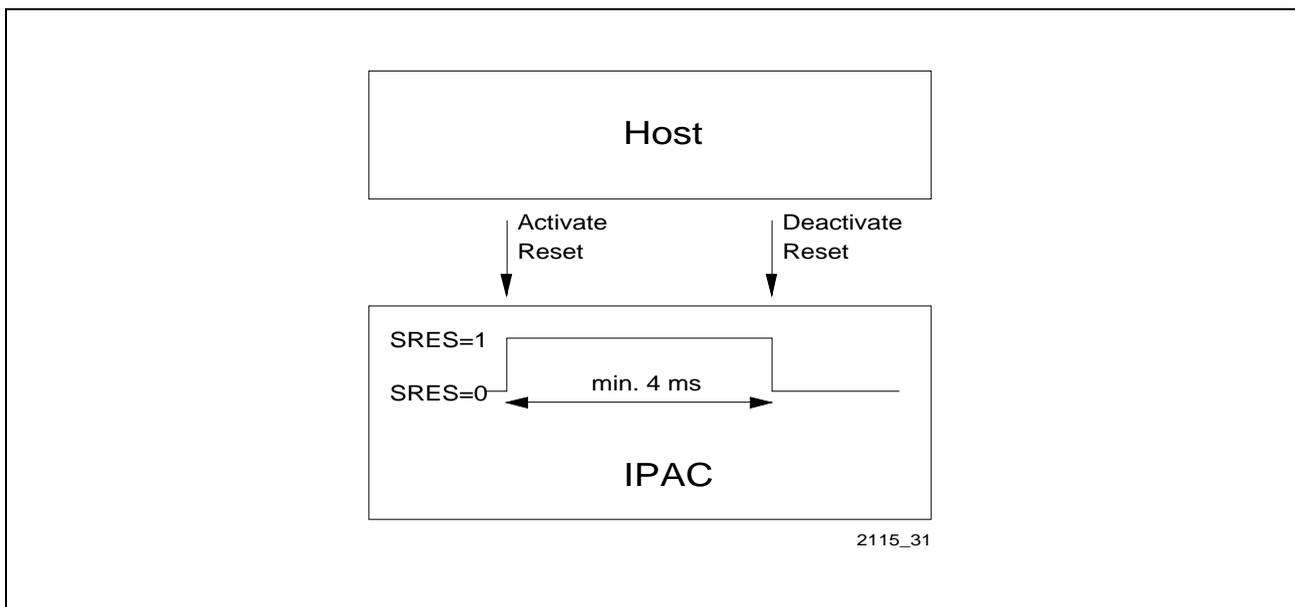
Figure 50 Reset Timing
