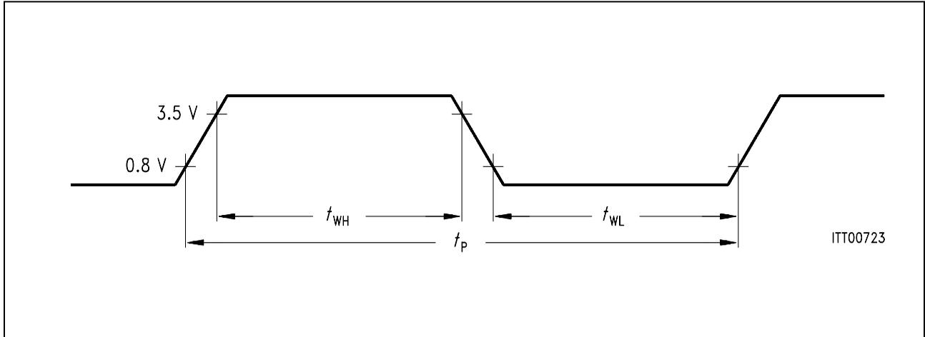
**Figure 116 Definition of Clock Period and Width**
