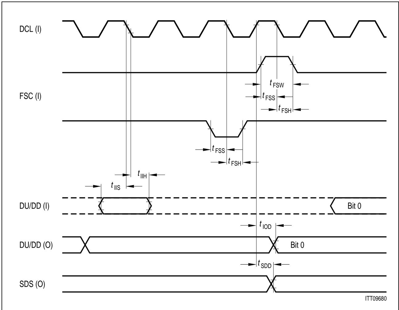
Figure 111 IOM<sup>®</sup> Timing (LT-S, LT-T mode)
