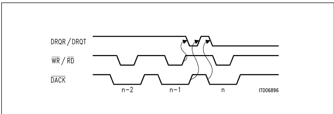
**Figure 45** DMA-Transfers with Pulsed  $\overline{DACK}$  (read or write)
