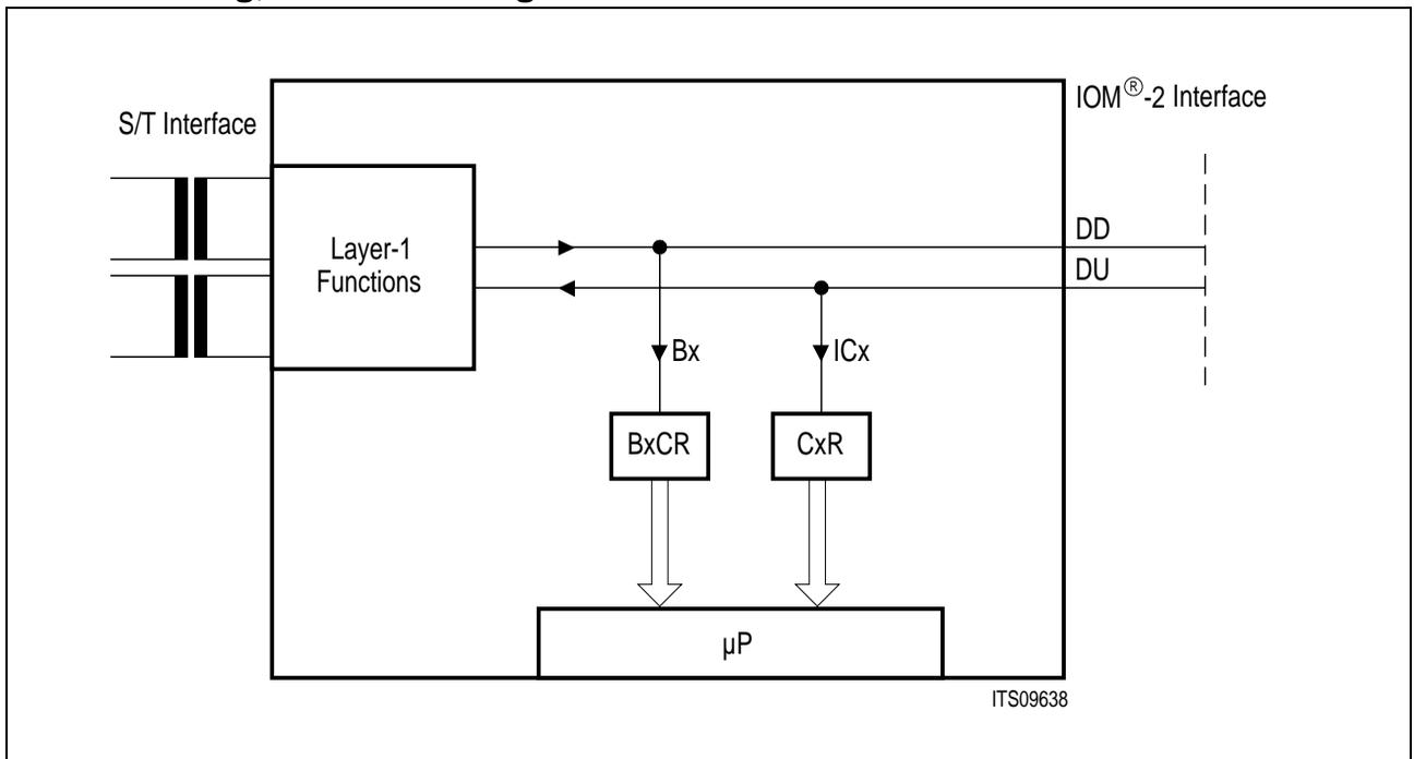
Figure 61 Access to B and IC Channels in IOM<sup>®</sup>-2 Terminal Mode
