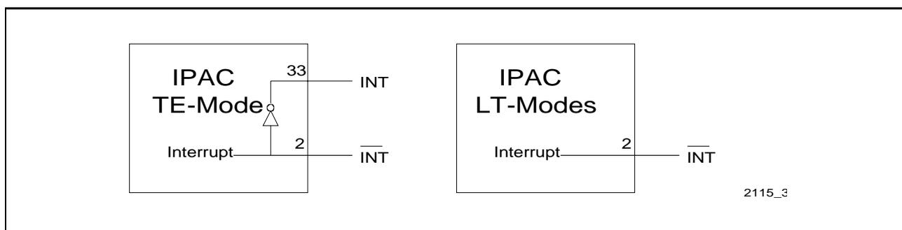
**Figure 38 High and Low Active Interrupt Output**
