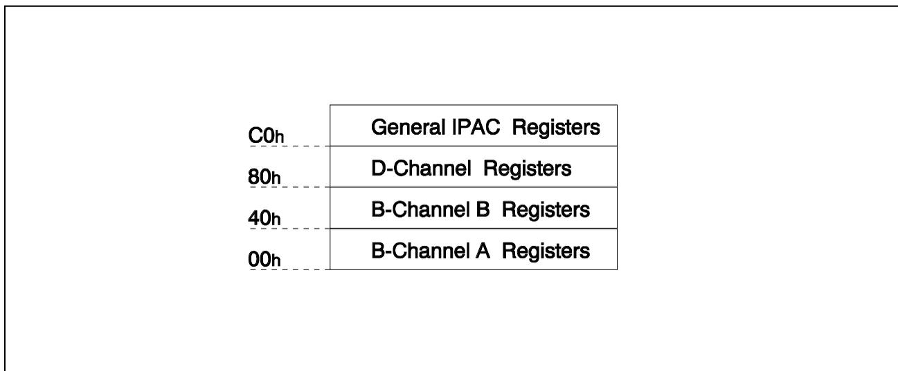
**Figure 98 Register Mapping**
