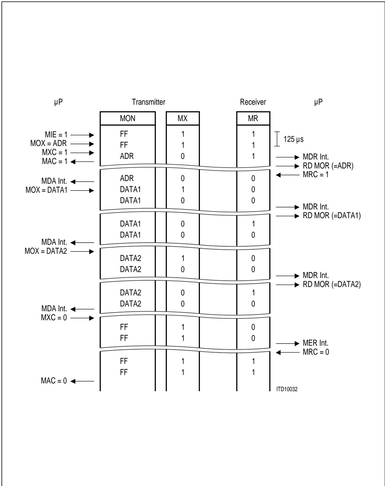
Figure 63 MONITOR Channel Protocol (IOM<sup>®</sup>-2)
