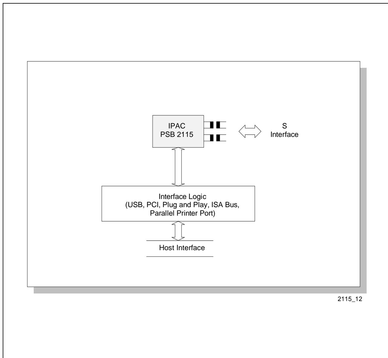
**Figure 4 ISDN PC Adapter Card for S Interface**
