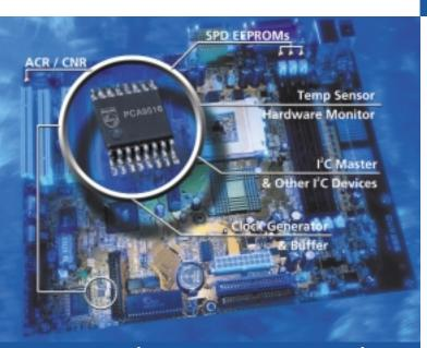
These bi-directional  $I^2C$  drivers enable designers to isolate the  $I^2C$  bus or SMBus capacitance into smaller sections, accommodating more devices or a longer bus length. Only 400 pF load is allowed on the bus and these devices break the  $I^2C$  bus or SMBus into multiple 400 pF segments.
