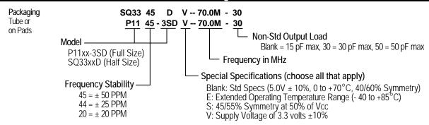
Consult factory for available frequencies and specs. Not all options available for all frequencies. A special part number may be assigned. Frequency Stability is inclusive of frequency shifts due to calibration, temperature, supply voltage, shock, vibration and load
