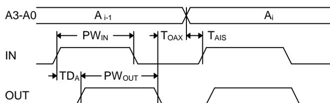
Figure 1: Timing Diagram
