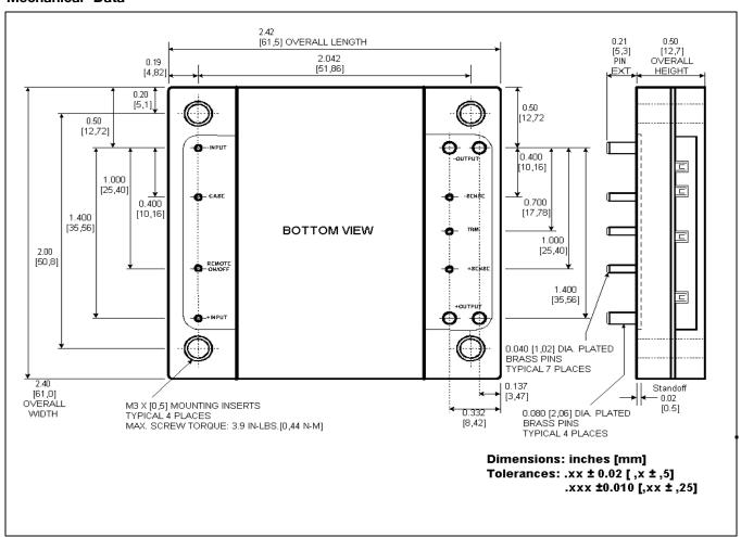
**PKL 4118A PIT (180W)**  $T_{C} = -40...+100^{\circ}C$ ,  $V_{I} = 36...75V_{dc}$  unless otherwise specified
