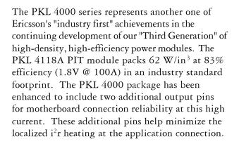
This product features fast dynamic response times and low output ripple, which are important parameters when supplying high quality DC power to Data Processing and Communications applications. The PKL 4000 Series also is
