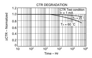
★ The measurement of TYPICAL CHARACTERISTICS are only for reference, not guaranteed.
