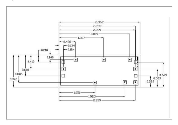
Die size: 2.36 x 0.94mm RF bond pads (1 & 5): 120 x 120 $\mu$ m All other bond pads: 120 $\mu$ m x 120 $\mu$ m Die Thickness: 100 $\mu$ m
