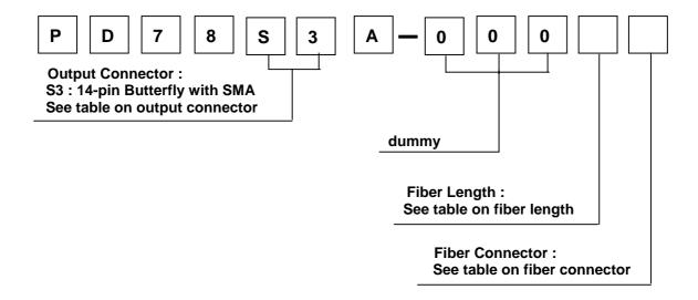
The standard product is 14-pin butterfly package with SMA(male or female) connector. Other types of connectors (GPO, K-connector) are also available upon request.
