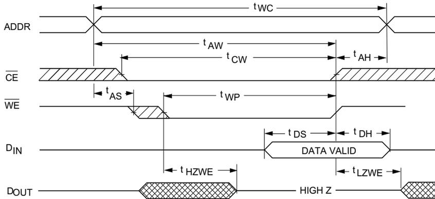
**Write Cycle No. 2 (Chip Enable Controlled)**
