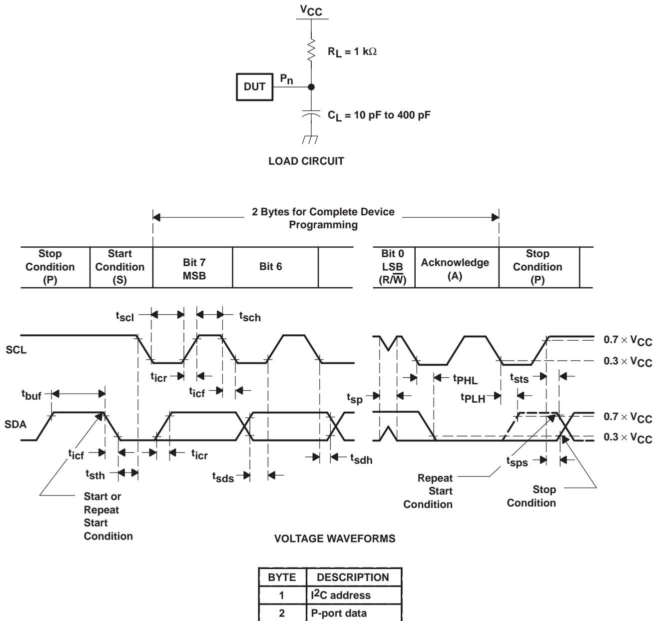
Figure 1. I<sup>2</sup>C Interface Load Circuit and Voltage Waveforms
