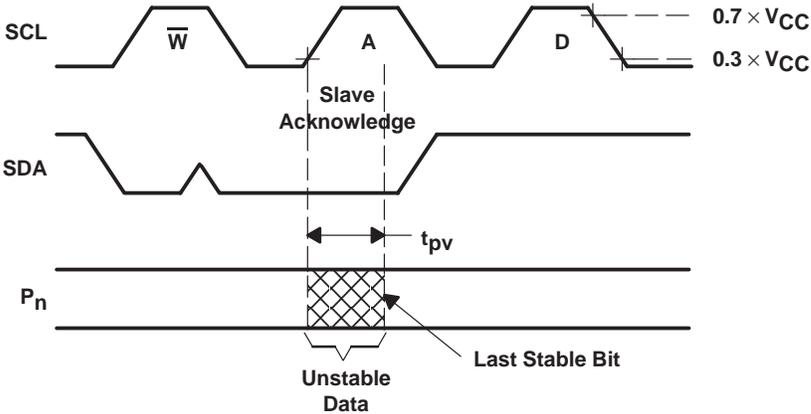
Figure 3. Write-Mode Timing
