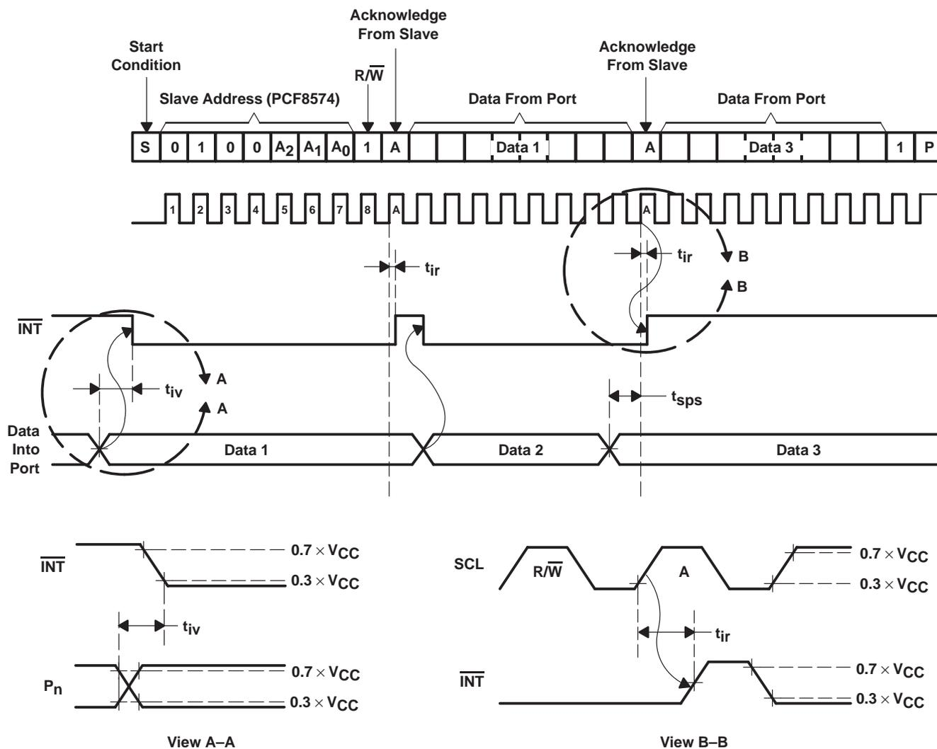
Figure 2. Interrupt-Timing Waveforms
