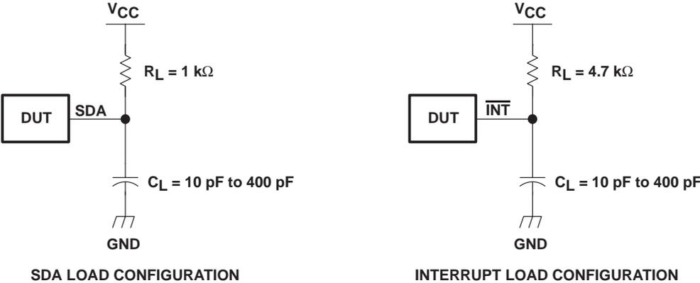
Figure 4. Load Circuits
