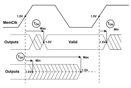
Table 15. 401GF Synchronous Output Timings
