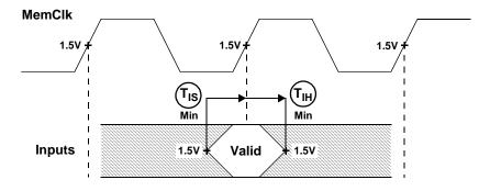
**Table 13. 401GF Synchronous Input Timings**
