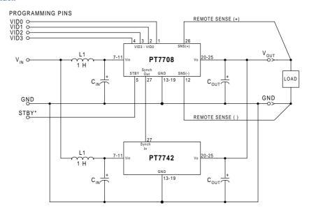
External Capacitors: The PT7742 requires a minimum ouput capacitance of 330µF for proper operation. The PT7742 also requires an input capacitance of 1500µF, which must be rated for a minimum of 1.4Arms of ripple current. For transient or dynamic load applications additional capacitance may be required. For more information refer to the application note regarding capacitor selection for this product.
