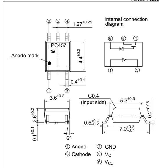
\* "OPIC"(Optical IC) is a trademark of the SHARP Corporation. An OPIC consists of a light-detecting element and signal-processing circuit integrated onto a single chip.
