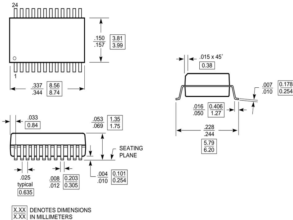
**24-Pin SOIC (S) Package Mechanicals**
