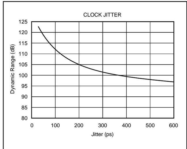
FIGURE 11. Jitter Sensitivity.
