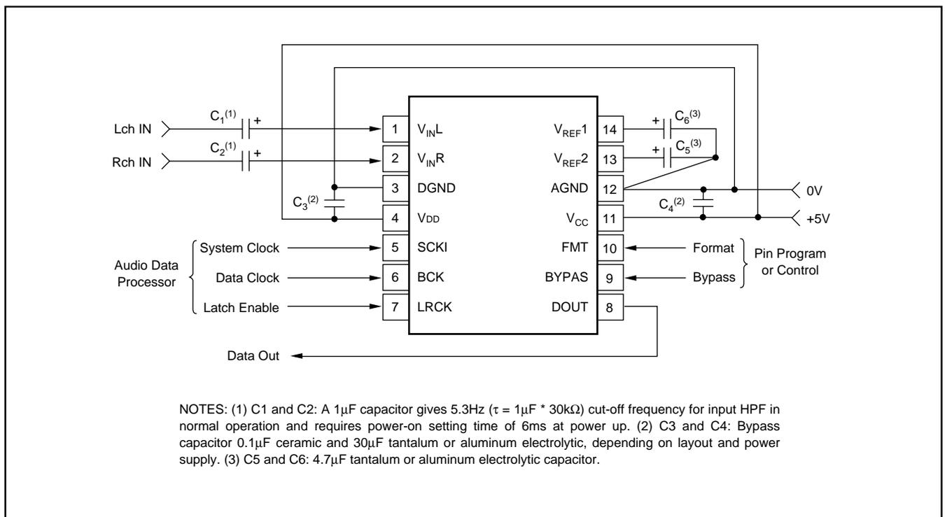
FIGURE 6. Typical Circuit Connection.
