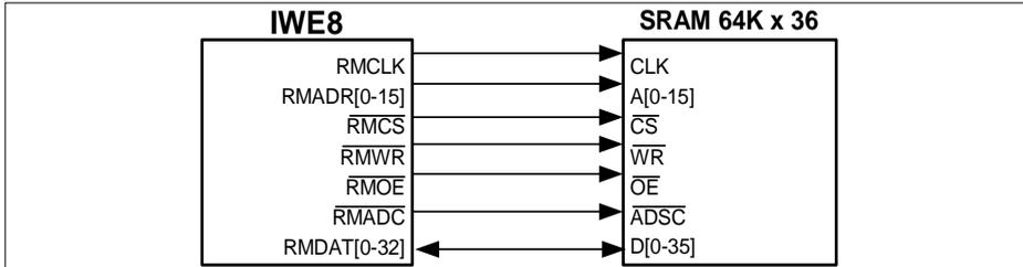
**Figure 34 External RAM Connection**
