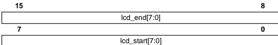
**lcd\_end**      End of LCD detect on port N
