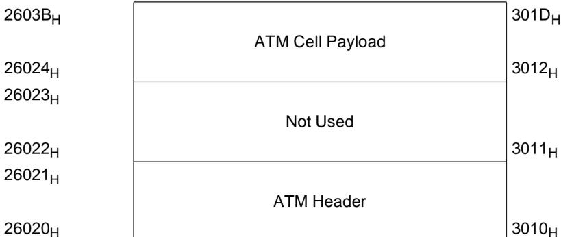
The ATM header to be used for cell insertion has to be programmed at MPADR = 26020<sub>H</sub>.
