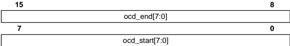
**ocd\_end** End of OCD (Out of cell delineation) state at port N
