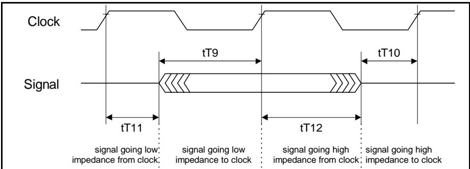
**Figure 65 Tri-state timing (multi-PHY, multiple devices only)**
