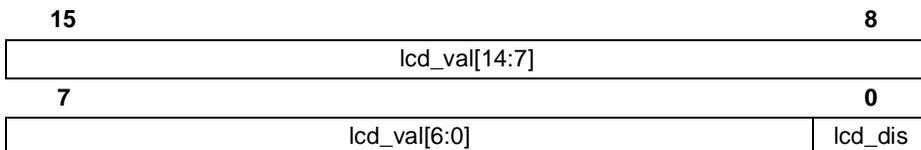
**lcd\_val**      LCD timer preload value
