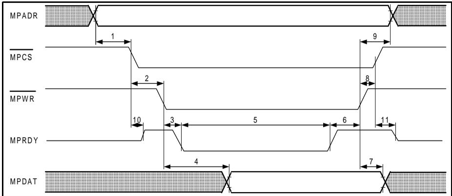
Figure 68 Intel Mode Write Cycle Timing Diagram
