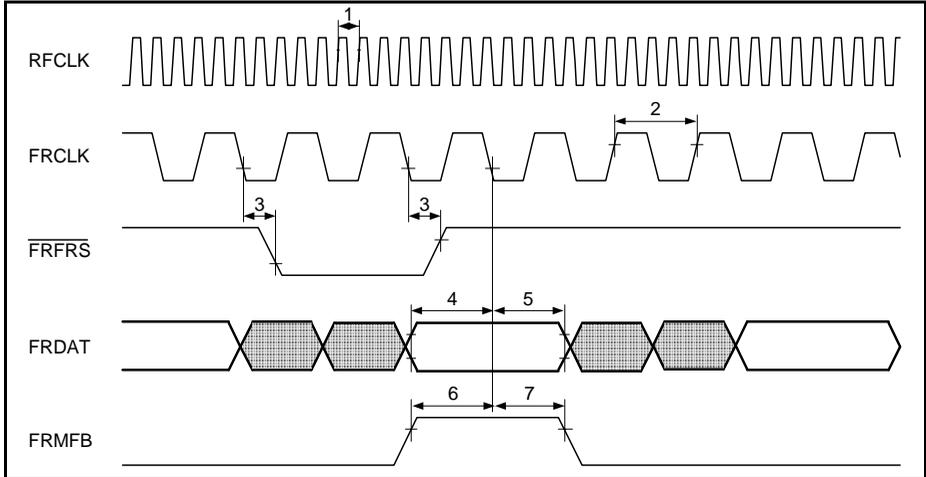
**Figure 57 Framer Receive Interface Timing in FAM**
