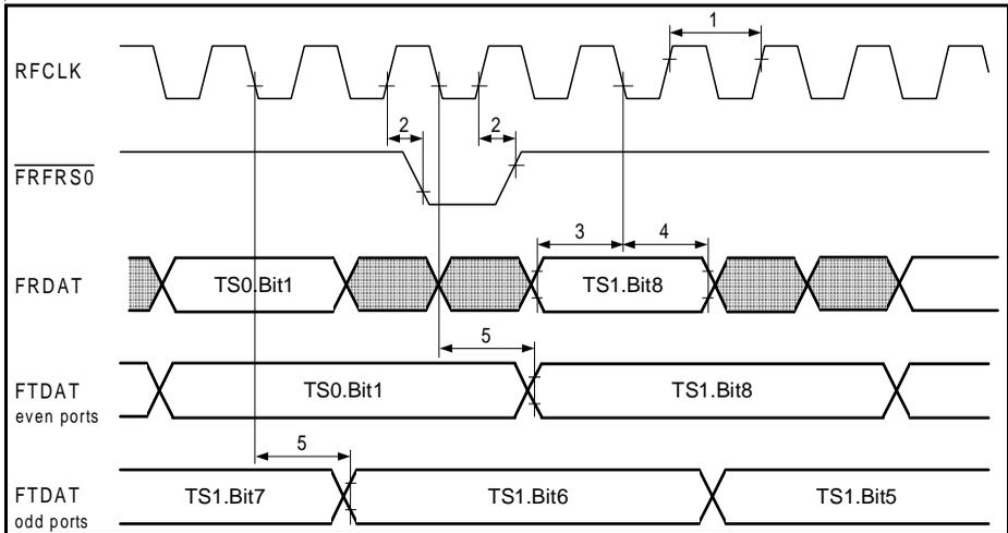
Figure 63 Framers Interface Timing in EC Mode
