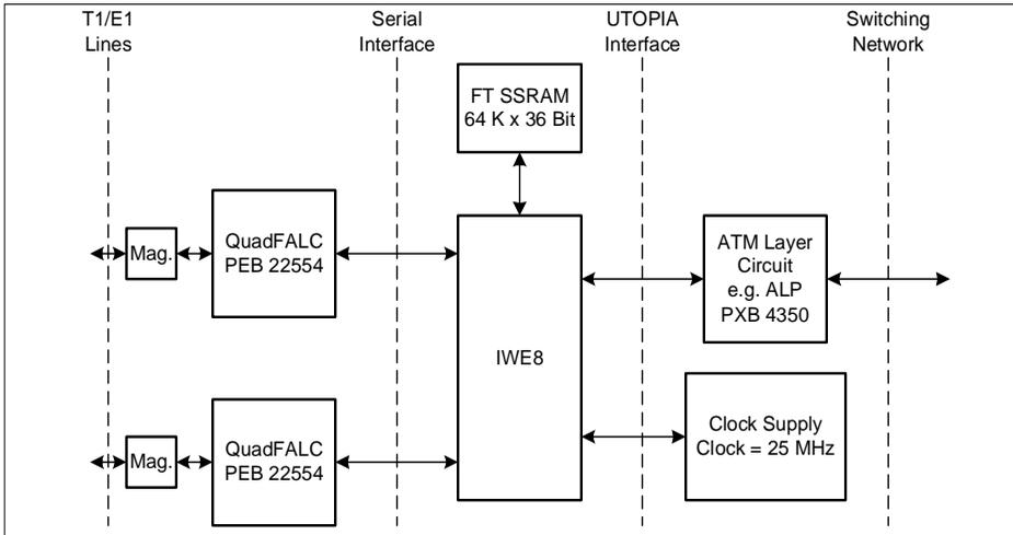
**Figure 3 Line Card for 8 T1/E1 Channels**
