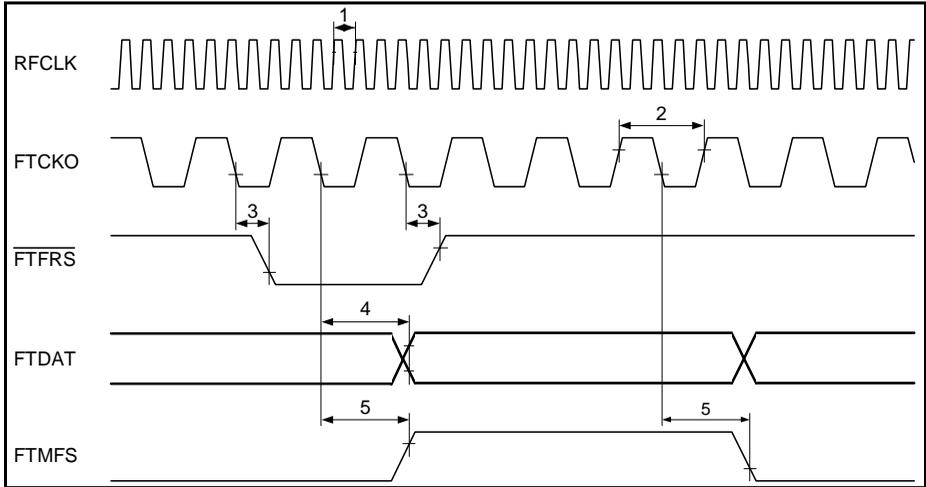
Figure 58 Framer Transmit Interface Timing in FAM
