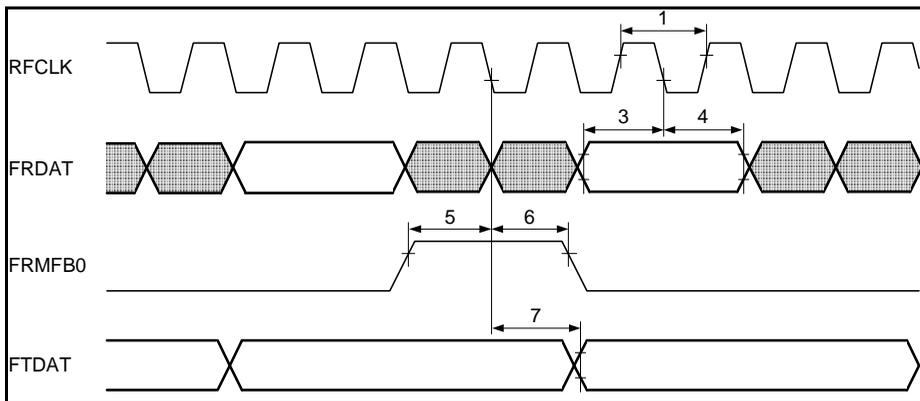
Figure 62 Framer Interface Timing in SYM 8.192 MHz
