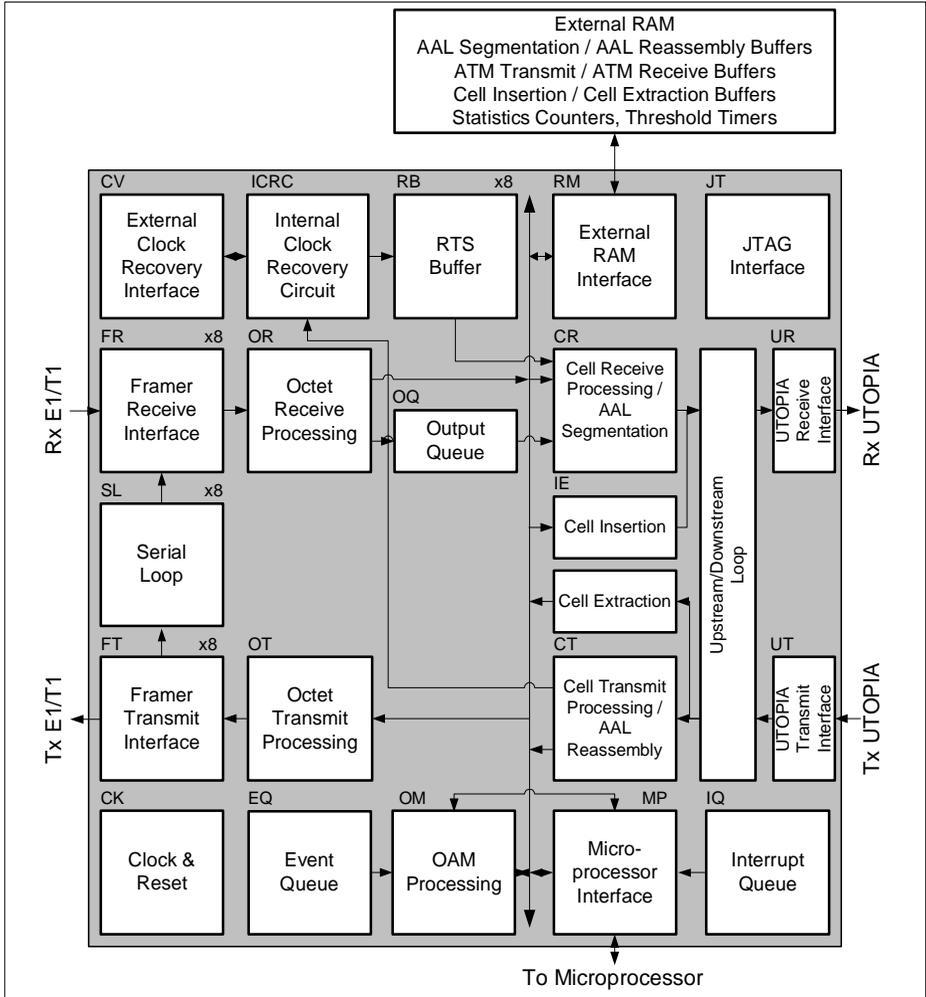
Figure 6 Block Diagram
