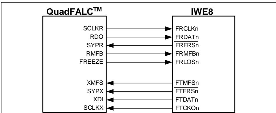
Figure 22 Connection of IWE8 to QuadFALC
