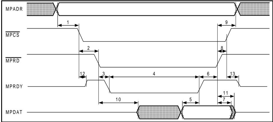
Figure 69 Intel Mode Read Cycle Timing Diagram
