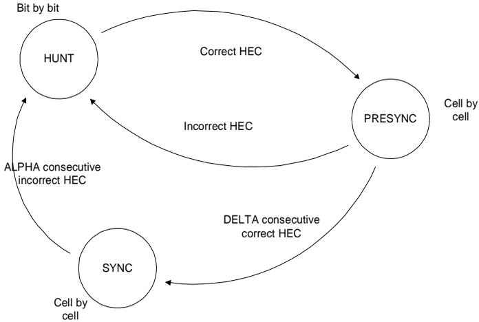
Note - The "correct HEC" means the header has no bit error (syndrome is zero) and has not been corrected
