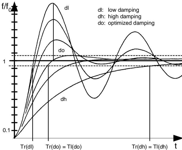
**Figure 21 Influence of Damping on Lock in Time**
