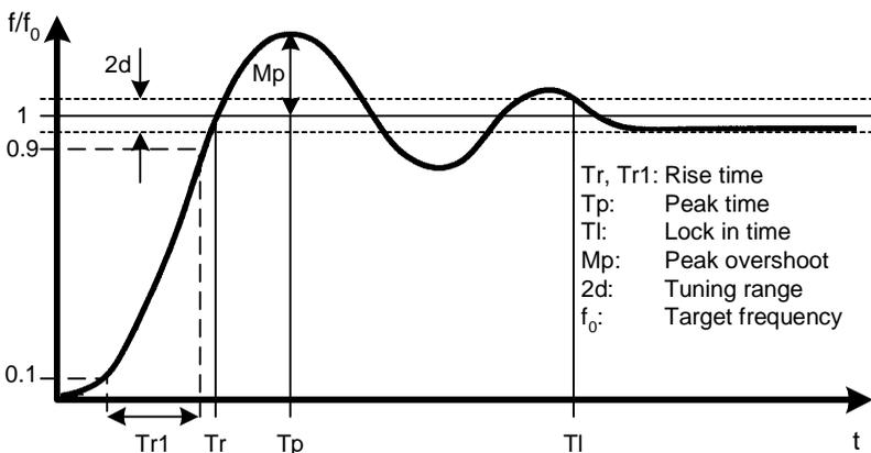
Figure 20 Transient Parameters
