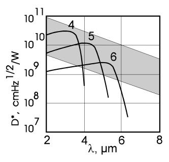
Spectral detectivity of PCI-4, -5 and -6 detectors.
