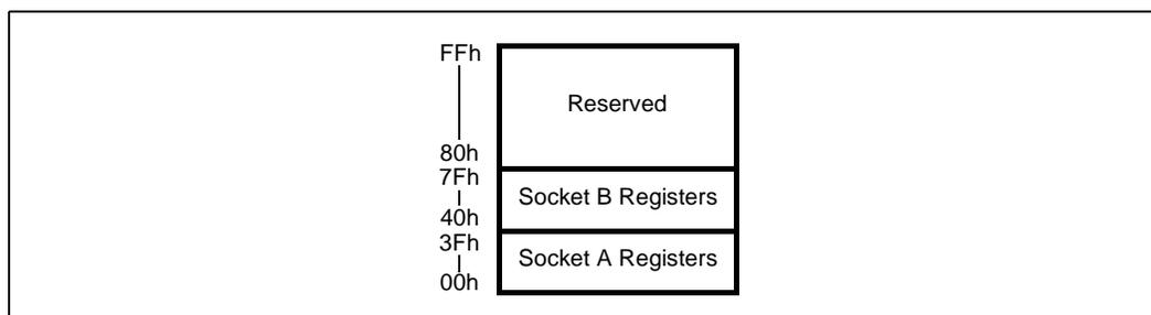
When viewed as a 7-bit value, the contents of this register completely specify a single internal-register byte. For example, when the value of this register is in the range 00h–3Fh, a Socket A register is selected (Socket Index bit is a ‘0’), and when the value of this register is in the range 40h–7Fh, a Socket B register is selected (Socket Index bit is a ‘1’).
