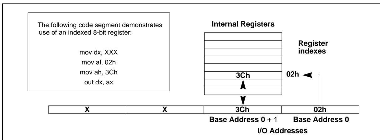
The PD6729 has Extension registers that add to the functionality of the 82365SL-compatible register set. Within the Extension registers is an **Extended Index** register and **Extended Data** register that provide access to more registers. The registers accessed through **Extended Index** and **Extended Data** are thus double indexed. The example below shows how to access the **Extension Control 1** register, one of the double-indexed registers.
