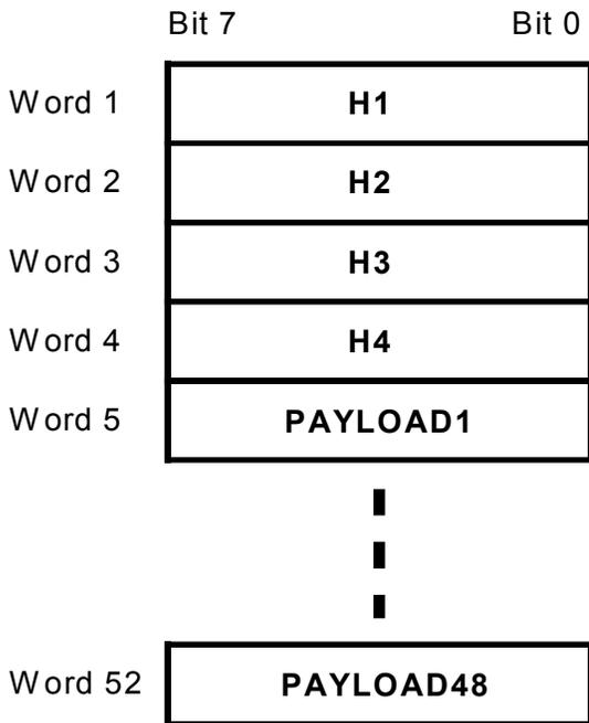
**Figure 19 8-bit Wide, 53-byte Word Structure**
