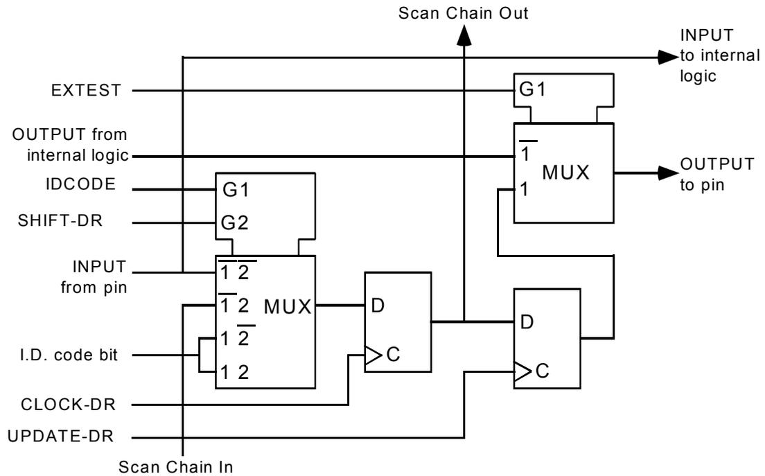
**Figure 28 Layout of Output Enable and Bi-directional Cells**
