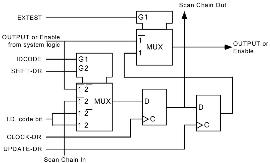
**Figure 27 Bi-directional Cell (IO\_CELL)**
