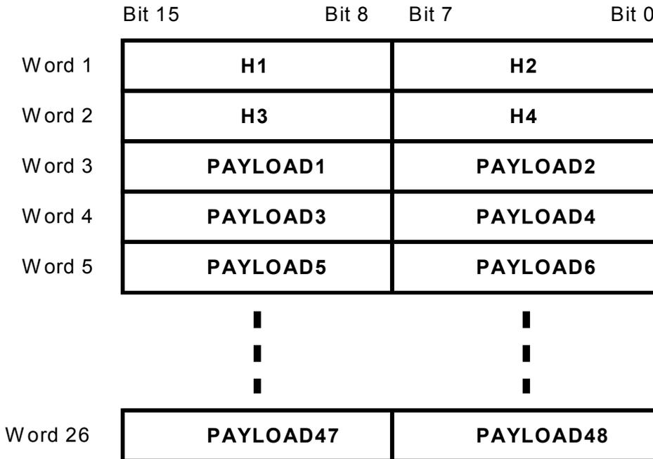
**Figure 17 16-bit Wide, 27-byte Word Structure**
