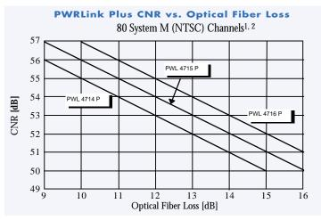
1. Specifications for 80 unmodulated System M (NTSC) channels and 200 MHz digital at -10 dBc. 2. Optical link defined as PWRLink Plus transmitter + 100% fiber link + HRM 3810 receiver.
