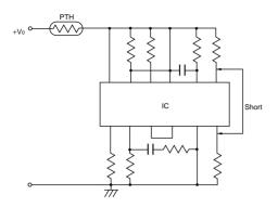
(4) Short-Circuit Test of Electrolytic Capacitor
