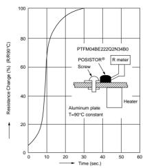
Relation between resistance change and time after POSISTOR® PTFM04BE222Q2N34B0 is installed on the part heated at a constant temperature of 90°C (3mm thick alminum sheet) is shown in the figure below.
