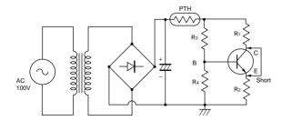
(2) Short-Circuit Test of Diode
