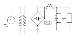
(5) Lock Test of Motor
