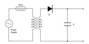
(2) Transformer Protection Circuit 2)
