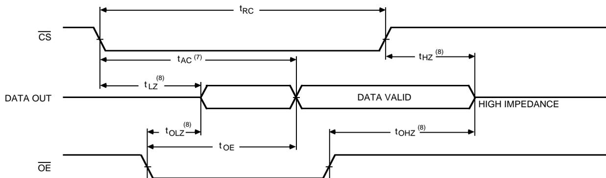
**Notes:**5.  $\overline{WE}$  is HIGH for READ cycle.6.  $\overline{CS}$  and  $\overline{OE}$  are LOW for READ cycle.7. ADDRESS must be valid prior to, or coincident with,  $\overline{CS}$  transition LOW,  $t_{AA}$  must still be met.8. Transition is measured  $\pm 200$  mV from steady state voltage prior to change, with loading as specified in Figure 1.
