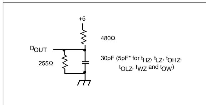
**Figure 1. Output Load**
