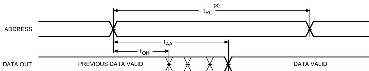
**TIMING WAVEFORM OF READ CYCLE NO. 2<sup>(6)</sup>**
