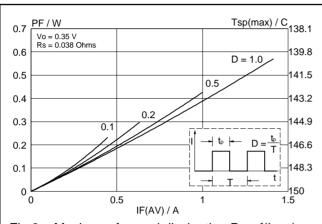
Fig.2. Maximum forward dissipation  $P_F = f(I_{F(AV)})$  per diode; square current waveform where  $I_{F(AV)} = I_{F(RMS)} x \sqrt{D}$ .
