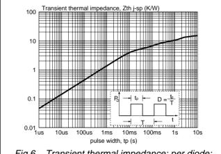
Fig.6. Transient thermal impedance; per diode;  $Z_{th j ext{-}sp} = f(t_p)$ .
