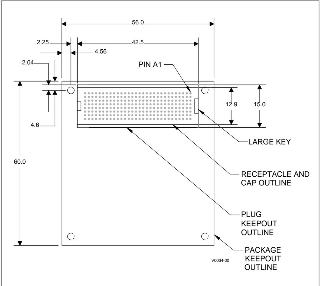
Figure 5.5. Mini-cartridge Assembly and Connector Keep-out Location, Top View (in mm)
