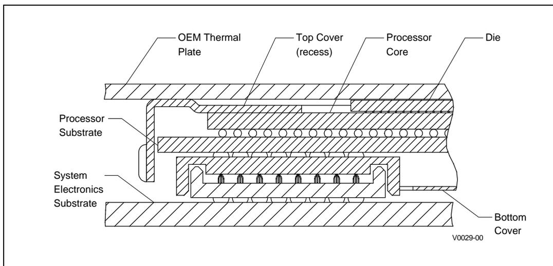
**Figure 5.1 Mini-cartridge Cross Section View**
