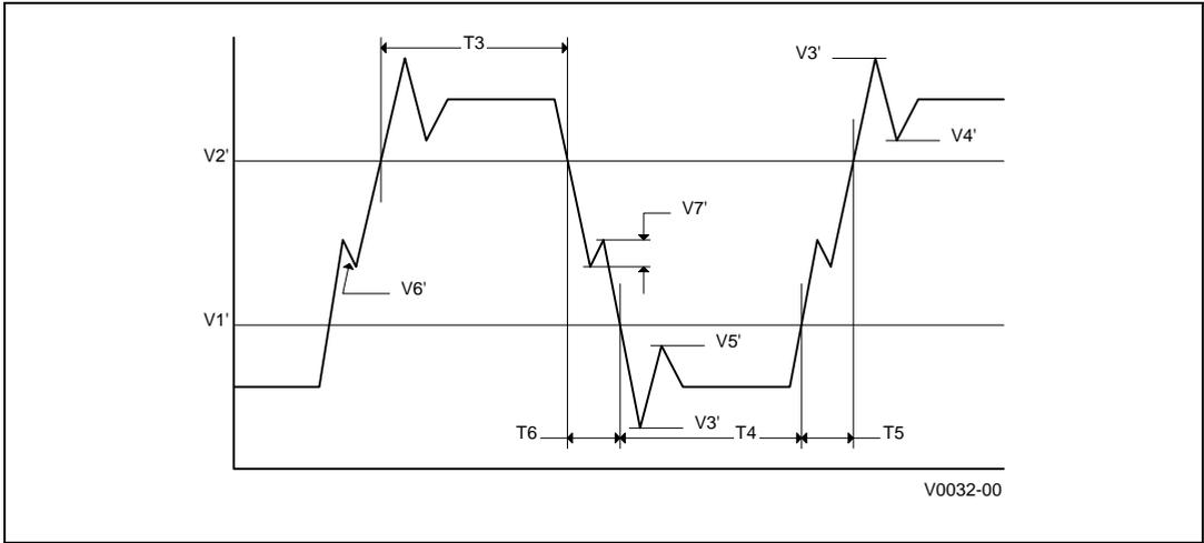
Figure 4.2 BCLK Generic Clock Waveform at the Processor Connector
