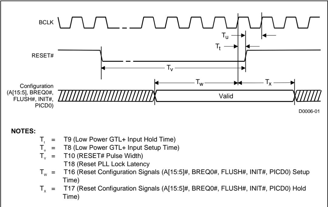
Figure 3.6 Reset and Configuration Timings
