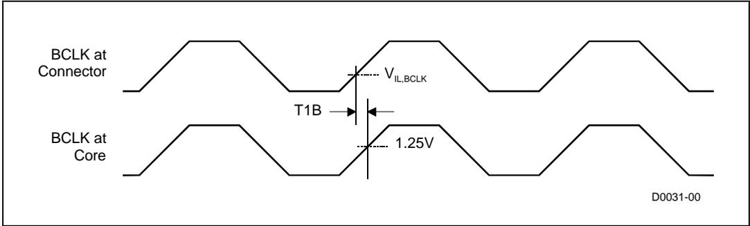
Figure 3.2 BCLK Connector to Core Offset
