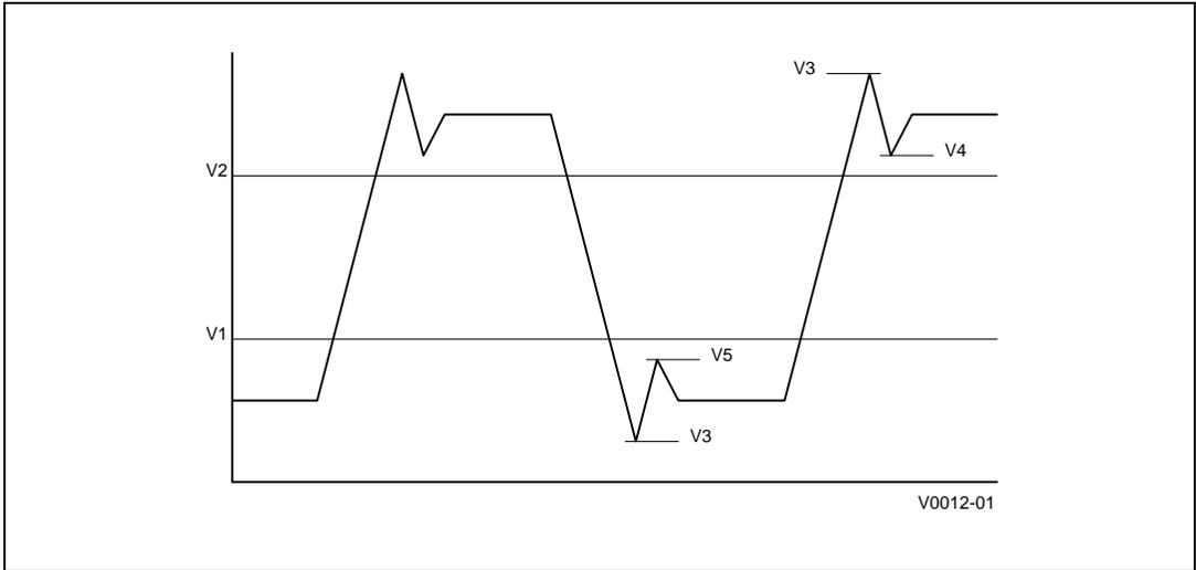
Figure 4.1 BCLK Generic Clock Waveform at the Processor Core
