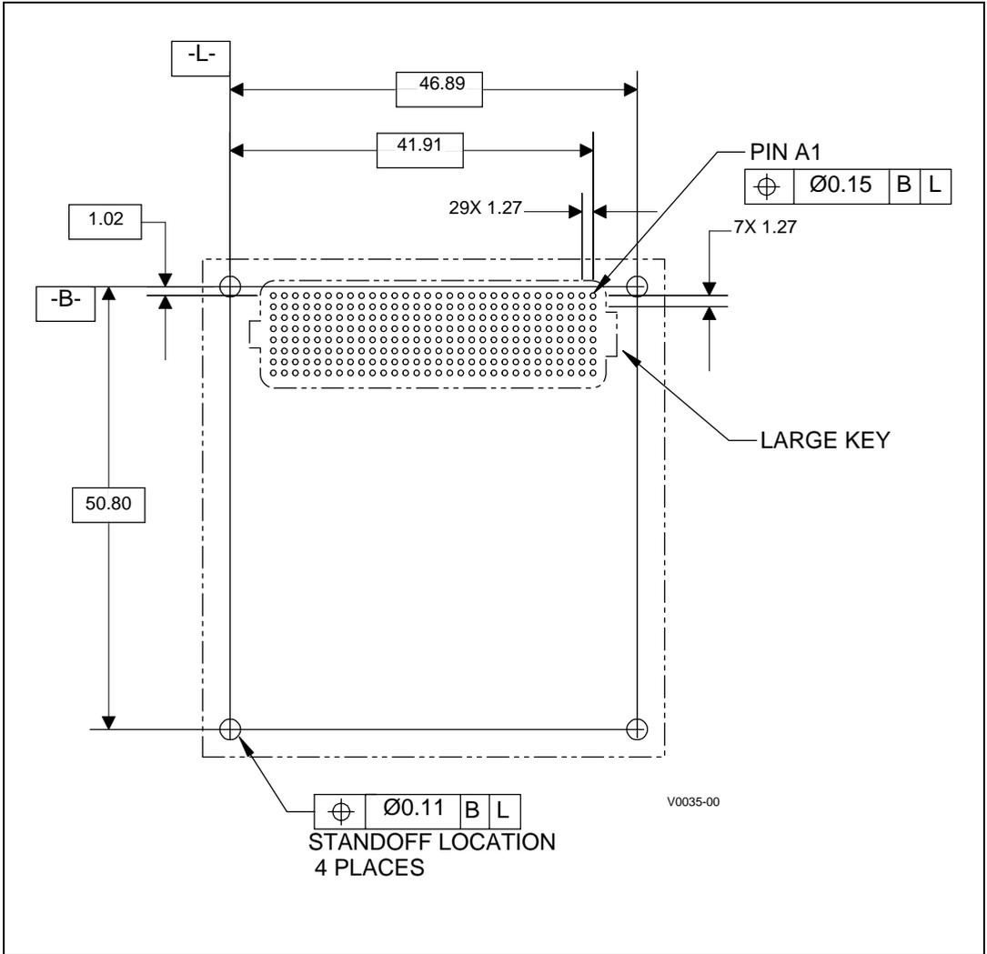
Figure 5.4 Standoff and Connector Location, Top View (in mm)
