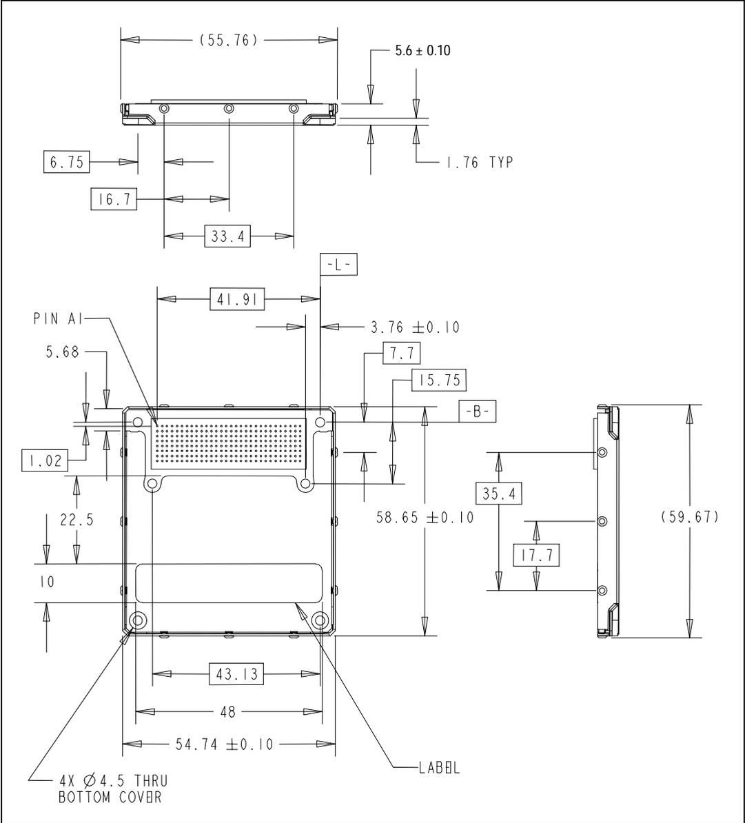
Figure 5.3 Mini-cartridge Assembly, Bottom Cover and Sides (in mm)
