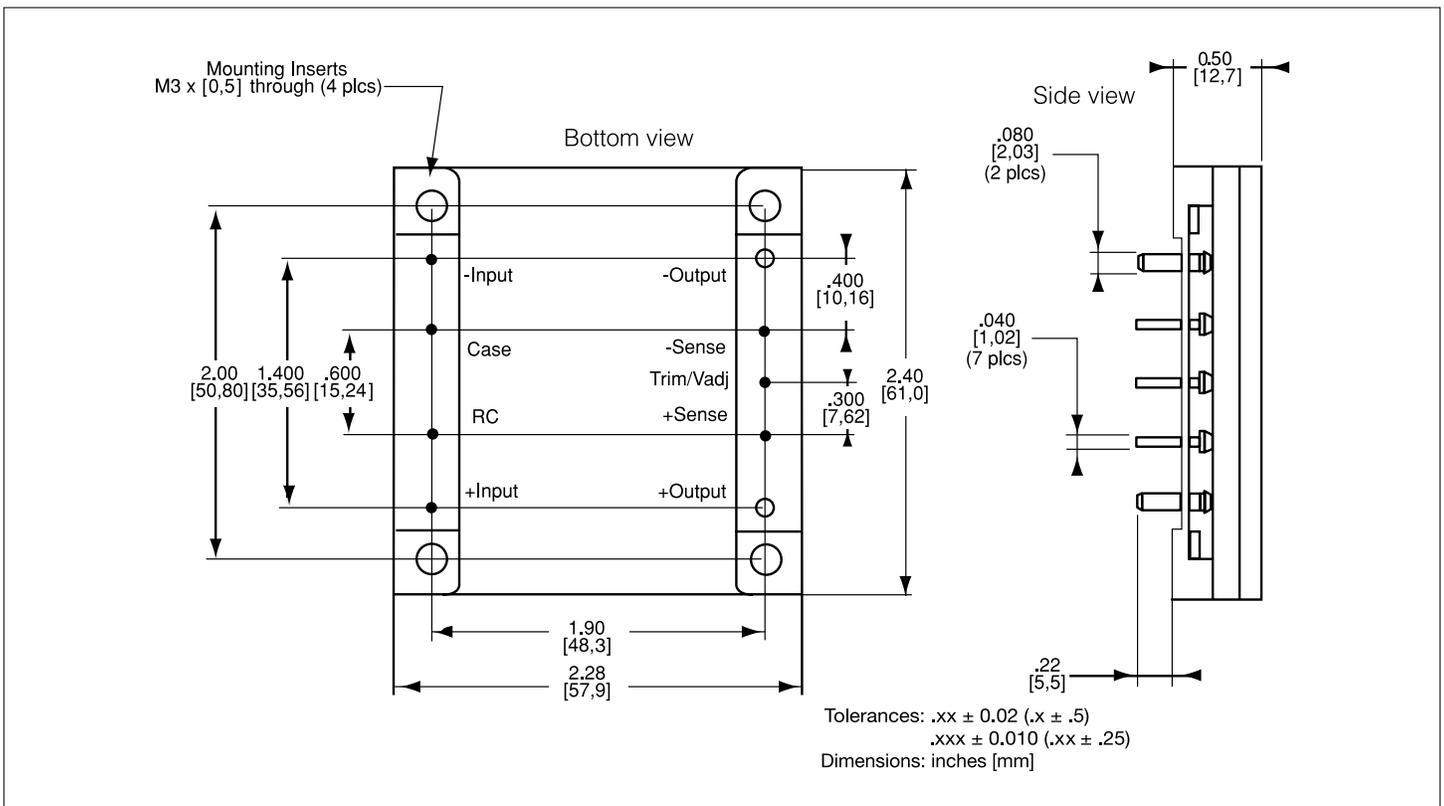
**PKJ 4518 PIT/PKJ 4318 PIT/PKJ 4218 PIT**  $T_C = -40...+100^{\circ}\text{C}$ ,  $V_I = 36...75\text{ V}$  dc unless otherwise specified.
