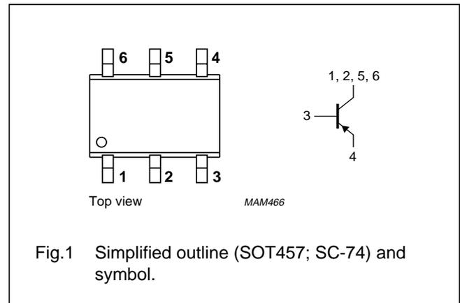
20 V low  $V_{CEsat}$  PNP transistor
