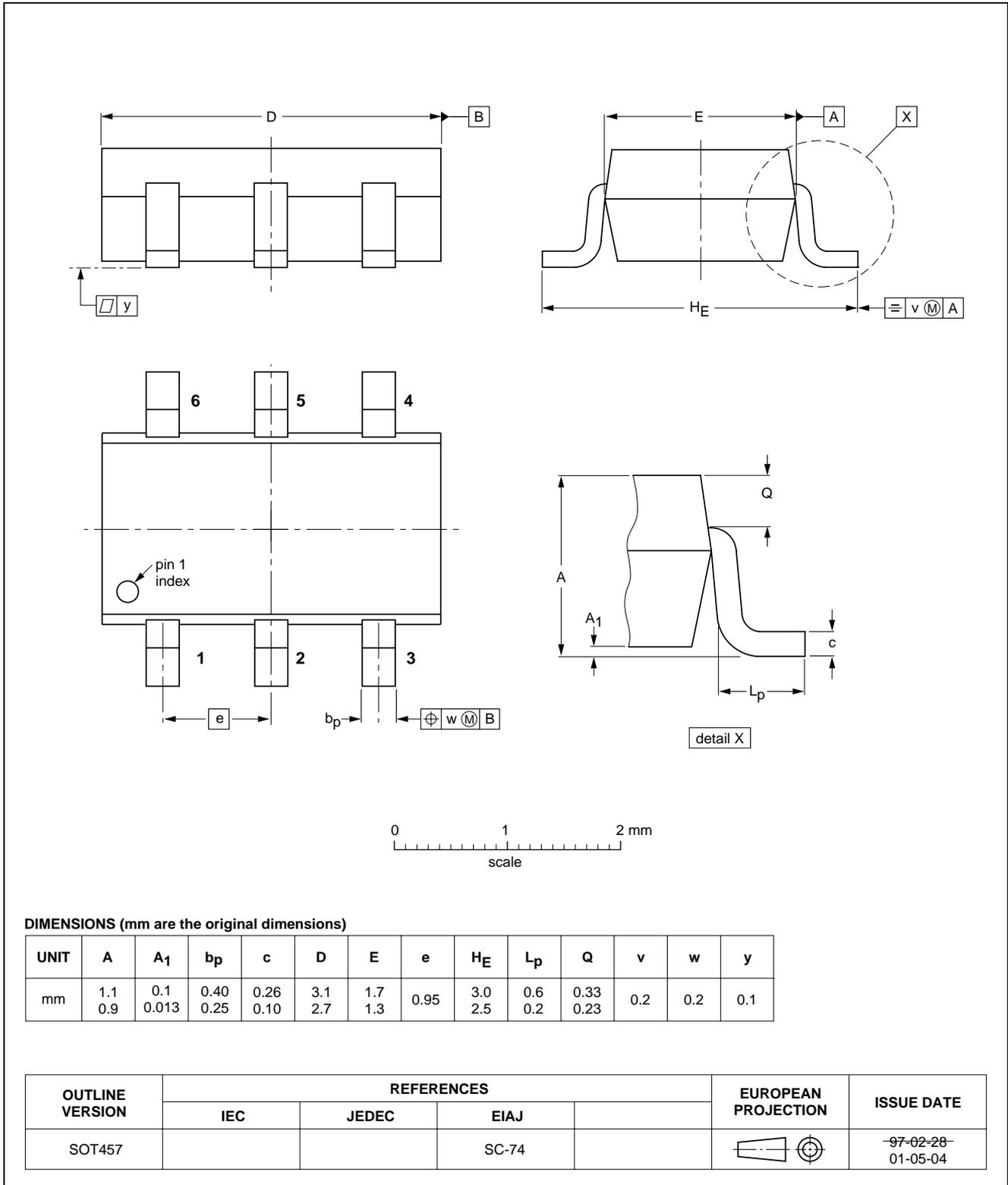
20 V low  $V_{CEsat}$  PNP transistor
