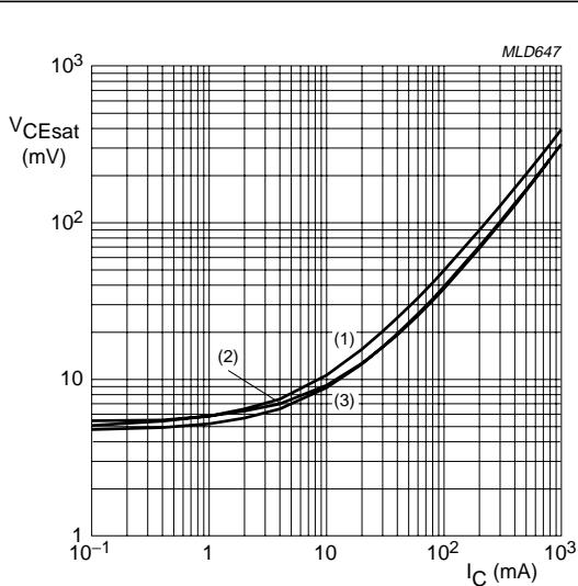
Fig.4 Collector-emitter saturation voltage as a function of collector current; typical values.
