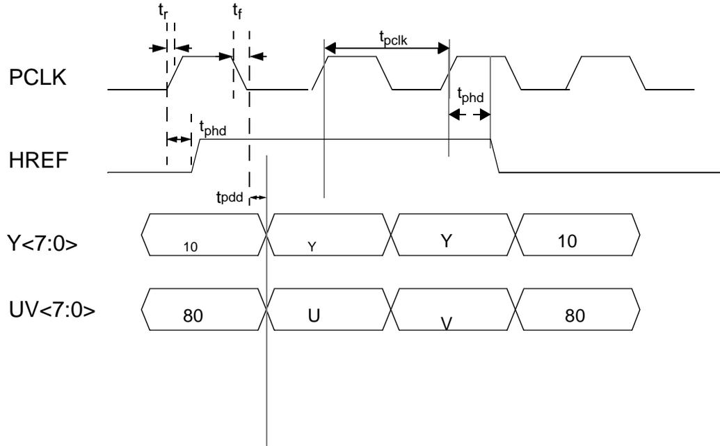
**FIG 2.2 Pixel Timing**
