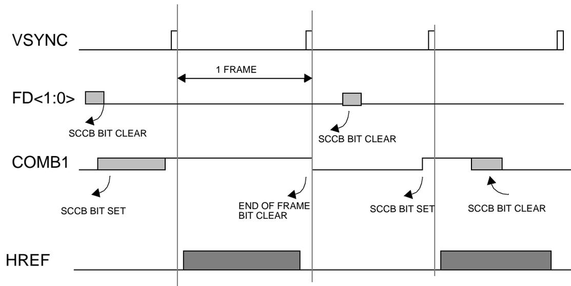
**FIG 1.8 Single Frame Transfer Example (Progressive Scan Mode)**
