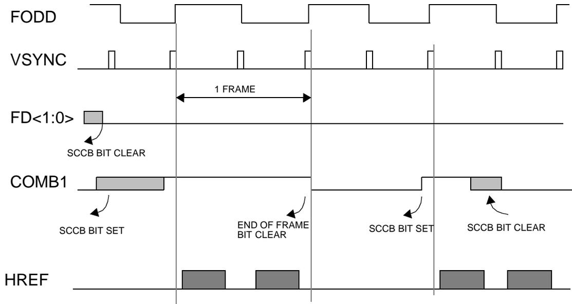
**FIG 1.7 Single Frame Transfer Example (Interlaced Mode)**
