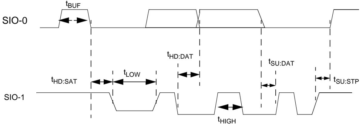
**FIG 2.3 SCCB Bus Timing**
