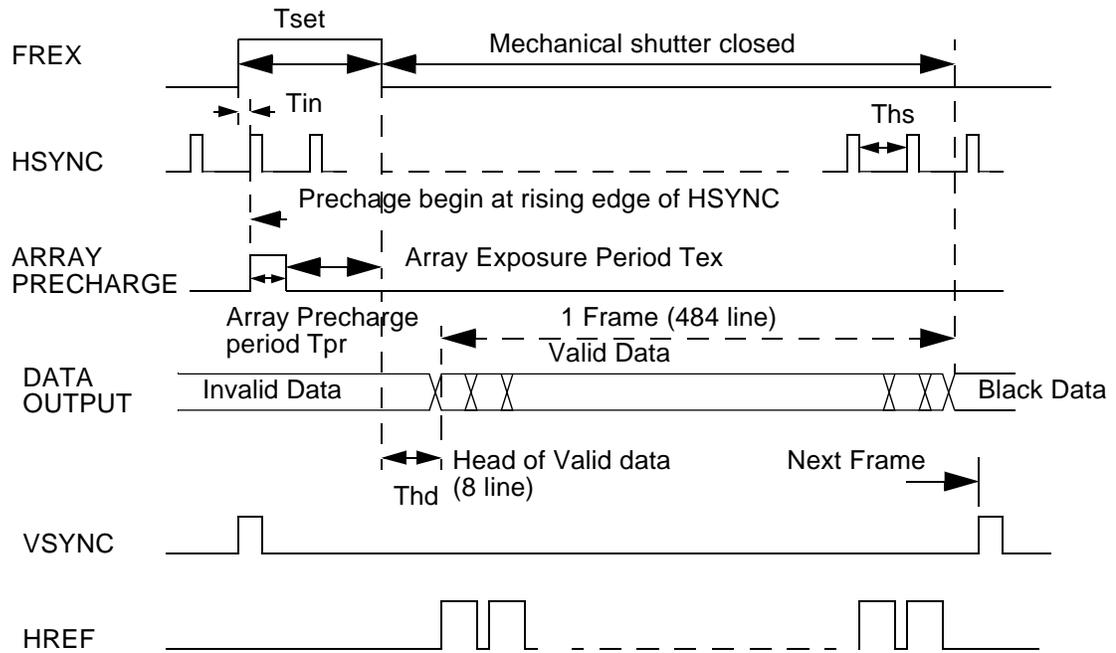
**FIG 1.6 Frame Exposure Timing**
