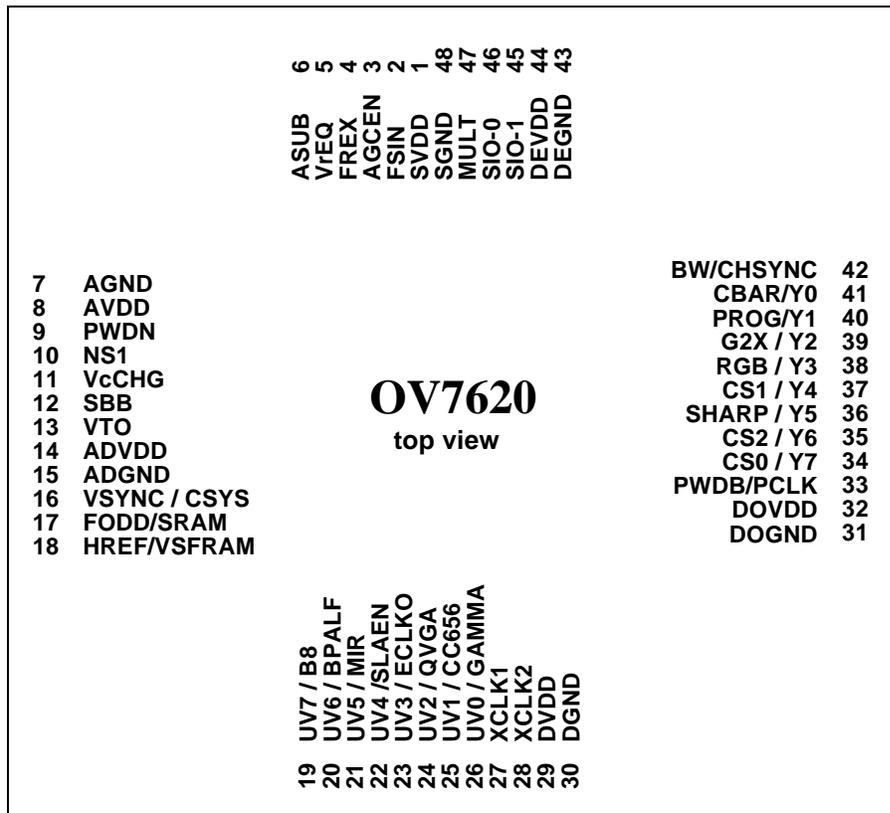
FIG 2.1 OV7620 48Pin Digital Package
