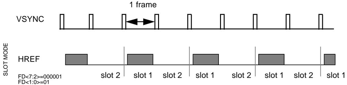
**FIG 1.10 Frame Division Examples (Progressive Scan Mode)**
