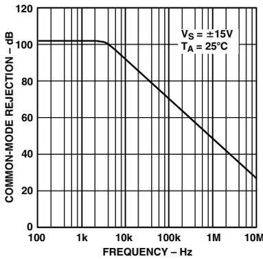
TPC 7. Common-Mode Rejection vs. Frequency
