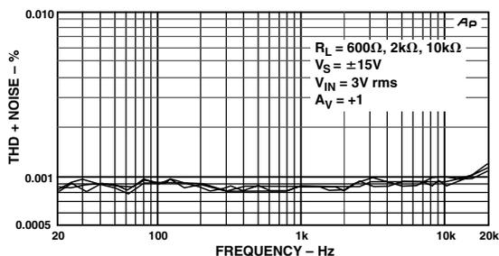
Figure 2. THD + Noise vs. Frequency vs.  $R_{LOAD}$
