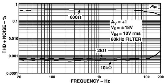
Figure 3. THD + Noise vs.  $R_{LOAD}$ ;  $V_{IN} = 10\ \text{V rms}$ ,
