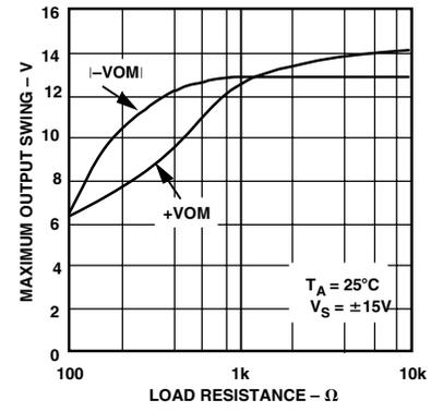
TPC 12. Maximum Output Voltage vs. Load Resistance
