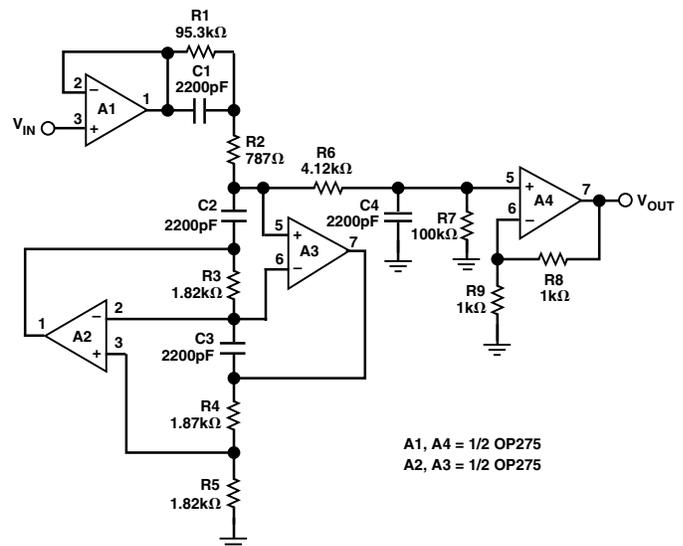
Figure 18. A 3-Pole,  $40\text{ kHz}$  Low-Pass Filter
