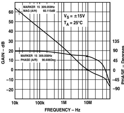
TPC 4. Open-Loop Gain, Phase vs. Frequency
