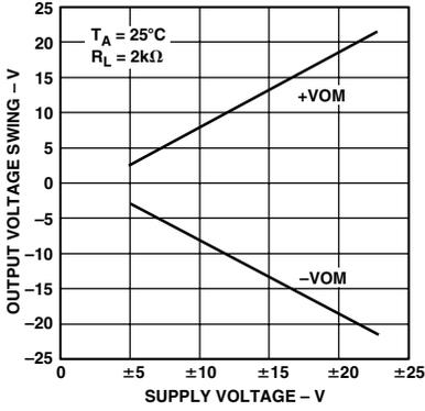
TPC 1. Output Voltage Swing vs. Supply Voltage
