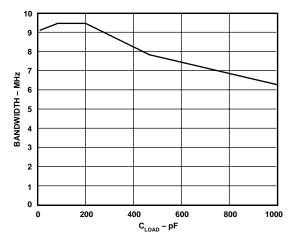
Figure 16. Bandwidth vs. CLOAD
