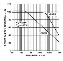
Power Supply Rejection vs. Frequency
