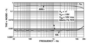
Figure 3. THD + Noise vs.  $R_{LOAD}$ ;  $V_{IN}$  =10 V rms,  $\pm$ 18 V Supplies
