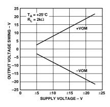
Output Voltage Swing vs. Supply Voltage
