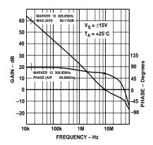
Open-Loop Gain, Phase vs. Frequency
