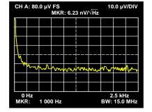
Small Signal Response  $R_L = 2 k\Omega$ ,  $V_S = \pm 15 V$ ,  $A_V = +1$
