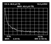
Figure 6. 1/f Noise Corner,  $V_S = \pm 15 \text{ V}$ ,  $A_V = 1000$
