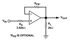
Figure 9. Output Voltage Phase Reversal Fix
