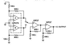
Figure 7. Noise Test Fixture
