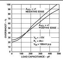
Small-Signal Overshoot vs. Load Capacitance
