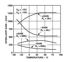
Open-Loop Gain vs. Temperature
