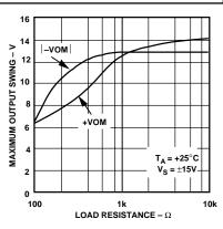
Maximum Output Voltage vs. Load Resistance
