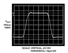
Figure 19. Low-Pass Filter Transient Response
