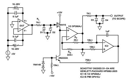
Figure 11. OP275's Settling Time Test Fixture
