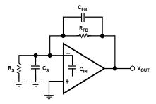
Figure 14. Compensating the Feedback Pole
