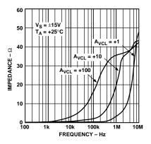
Closed-Loop Output Impedance vs. Frequency
