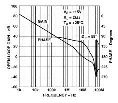
Open-Loop Gain, Phase vs. Frequency
