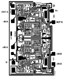
Die Size 0.070 × 0.108 in. (7,560 sq. mils) Substrate is connected to V-
