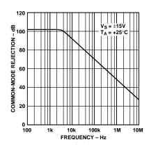
Common-Mode Rejection vs. Frequency
