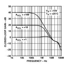
Closed-Loop Gain vs. Frequency
