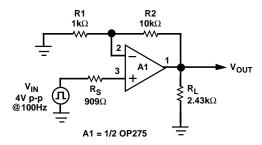
Figure 10. Overload Recovery Time Test Circuit
