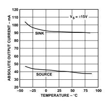
Short Circuit Current vs. Temperature
