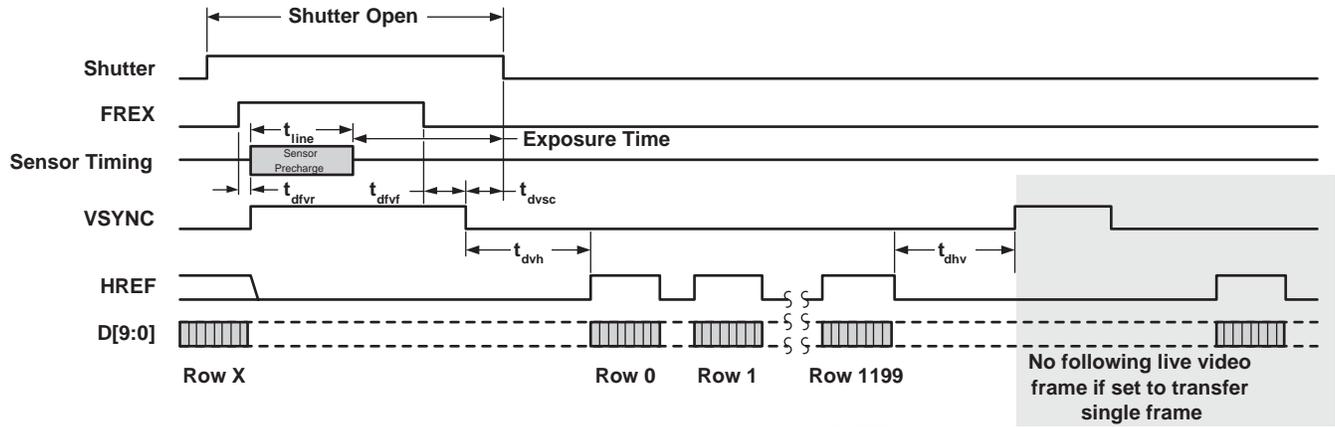
Figure 13 Frame Exposure Mode Timing with EXPSTB Asserted
