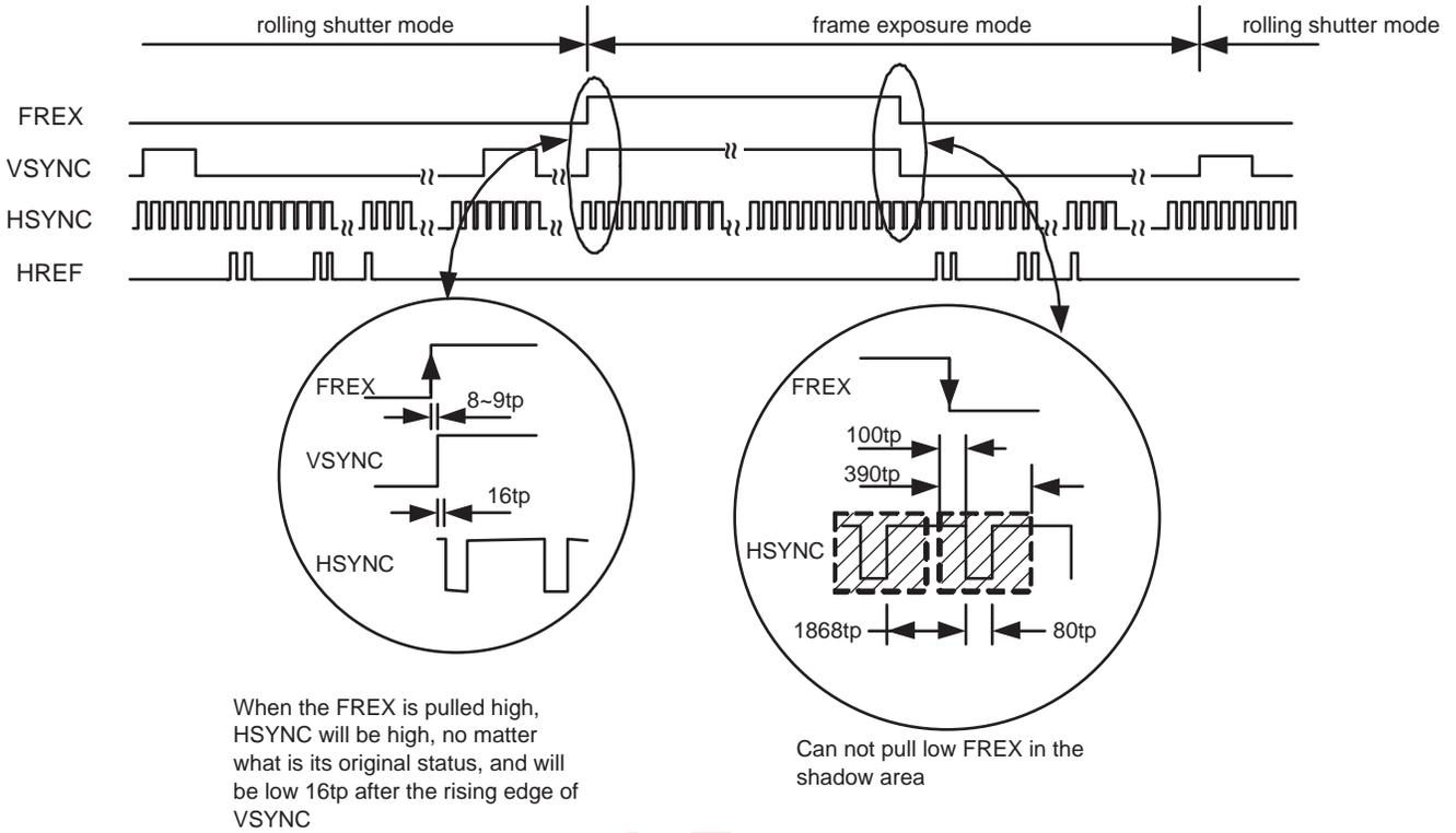
**Figure 15 Frame Exposure Mode Control Timing (SVGA Mode)**
