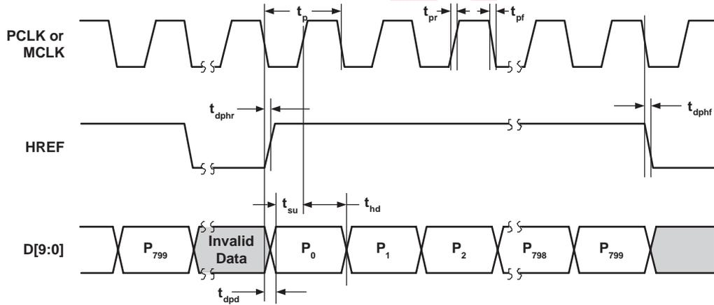
Figure 10 UXGA Frame Timing
