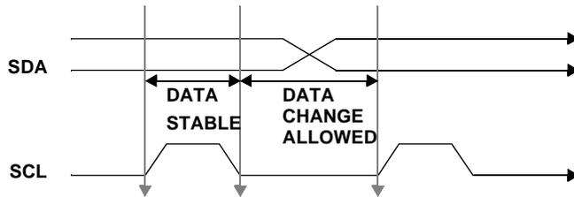
Figure 9. Bit Transfer on the I<sup>2</sup>C Bus
