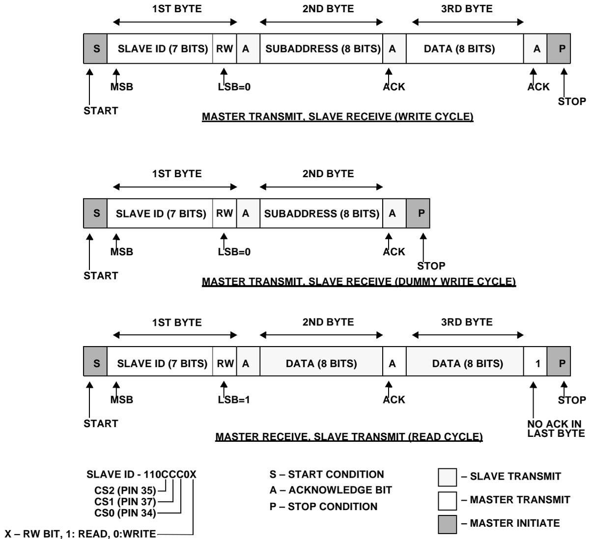
Figure 8. I<sup>2</sup>C Bus Protocol Format
