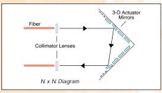
The electro-mechanical actuator design has linear control with overall <3dB insertion loss using the Blue Sky Research µLens™ to optimize fiber input/output collimation and coupling.
