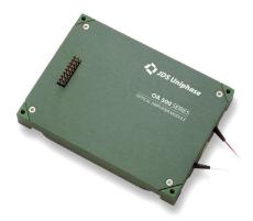
The JDS Uniphase OA 500 Amplifier Series provides C-band optical amplification in an economical and compact package. It is designed for use in dense wavelength division multiplexing (DWDM) telecommunication systems, at points where the signal is not multiplexed. It can also be used in edge or access networks, where gain flattening is not required.
