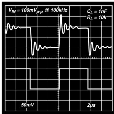
Figure 34. Output of OP250 without Snubber Network
