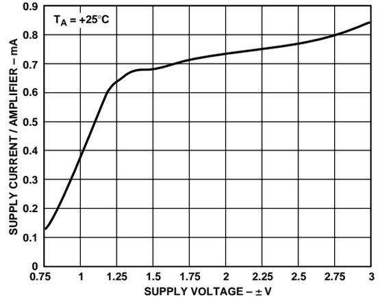
Figure 4. Supply Current per Amplifier vs. Supply Voltage
