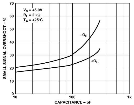
Figure 18. Small Signal Overshoot vs. Load Capacitance
