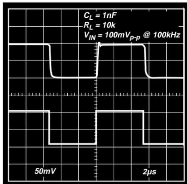
Figure 35. Output of OP250 with Snubber Network
