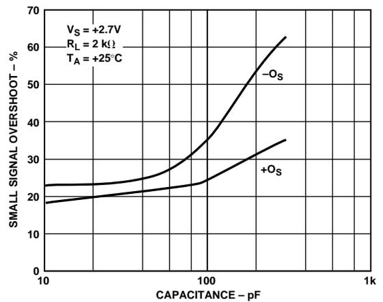
Figure 17. Small Signal Overshoot vs. Load Capacitance
