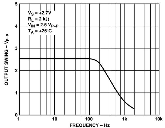
Figure 11. Closed-Loop Output Voltage Swing vs. Frequency
