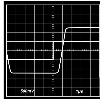
Figure 31. Saturation Recovery from the Negative Rail
