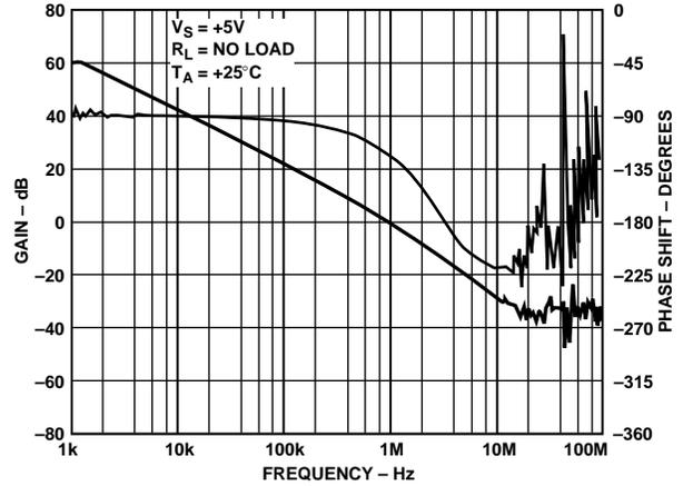
Figure 10. Open-Loop Gain and Phase
