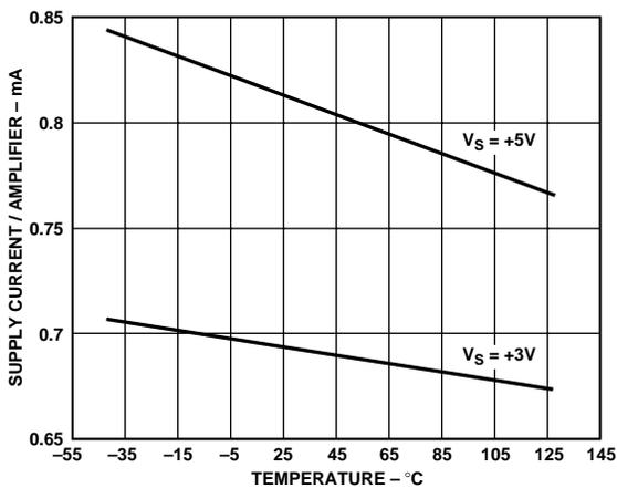
Figure 3. Supply Current per Amplifier vs. Temperature
