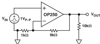
Figure 29. Overload Recovery Time Test Circuit
