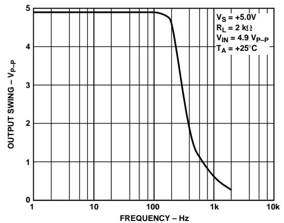
Figure 12. Closed-Loop Output Voltage Swing vs. Frequency
