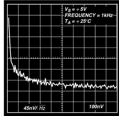
Figure 26. Voltage Noise Density vs. Frequency
