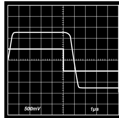
Figure 30. Saturation Recovery from the Positive Rail
