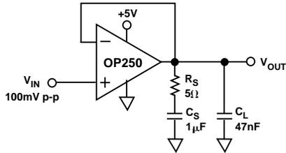
Figure 33. Schematic for Using a Snubber Network
