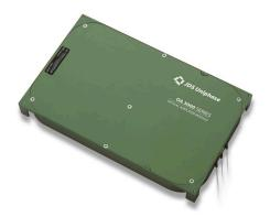
The JDS Uniphase OA 3000 Series is a controlled optical amplifier that features variable gain and transient suppression. The maximum optical output of 17 dBm and variable gain range of 10 dB to 25 dB make the module suitable for pre-amp, inline, or booster amplifier applications.
